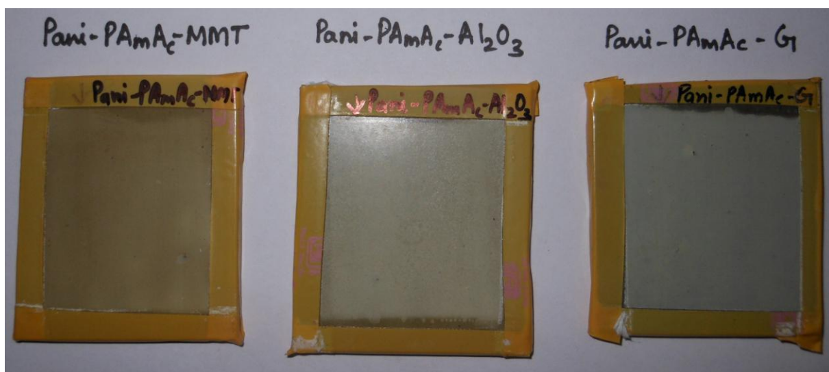
Fig. 4.69: Photographs of Pani-PAMAc-Nanoparticles/epoxy coatings after 2400 UV-weatherometer exposure
