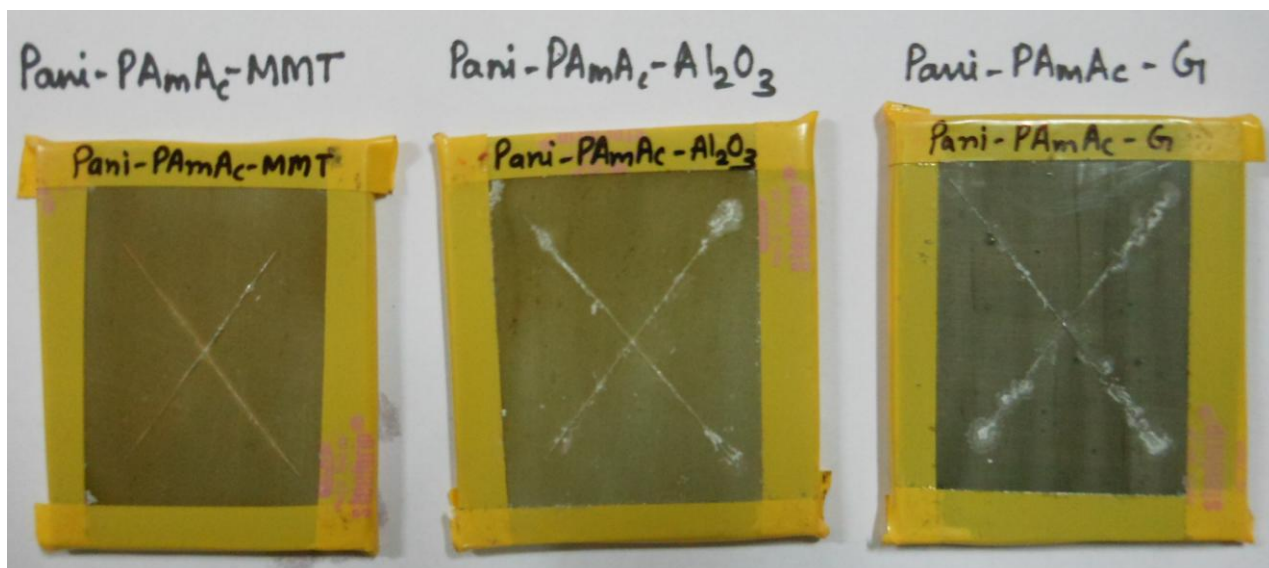
Fig. 4.68: Photographs of Pani-PAmAc-Nanoparticles/Epoxy coatings after 2400 h to salt spray exposure
