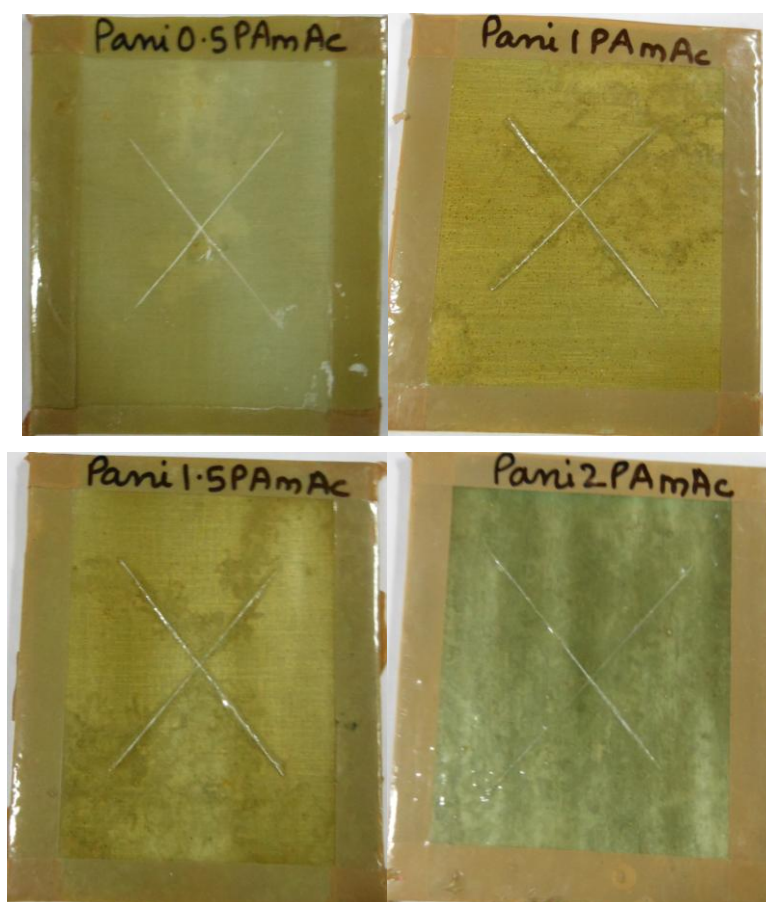
Fig. 4.47: Photographs of Pani-PAmAc/Epoxy coatings after 1200 h to salt spray exposure
