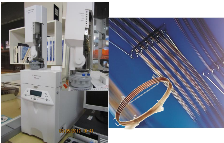
Figure 2.15. Agilent 6850 gas chromatograph (left) and Capillary column BP20 (right)
