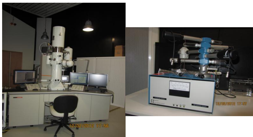
Figure 2.12. JEOL 2100F microscope (left) and single tilt specimen holder and vacuum pump (right)
