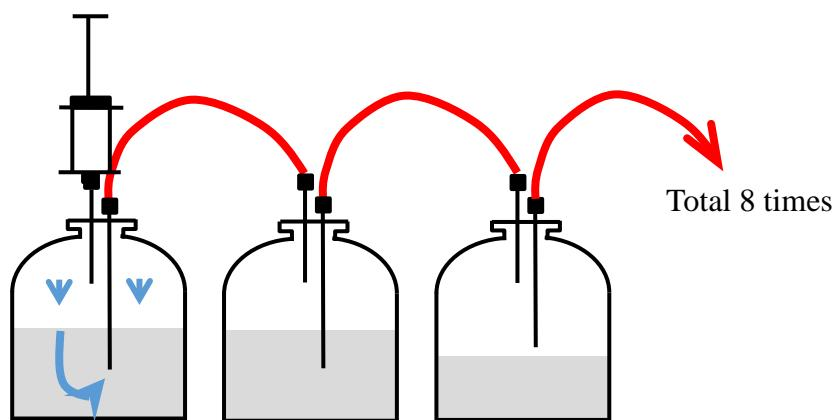
Figure 6a.1: Experimental setup for enrichment of H<sub>2</sub> producing bacteria.
