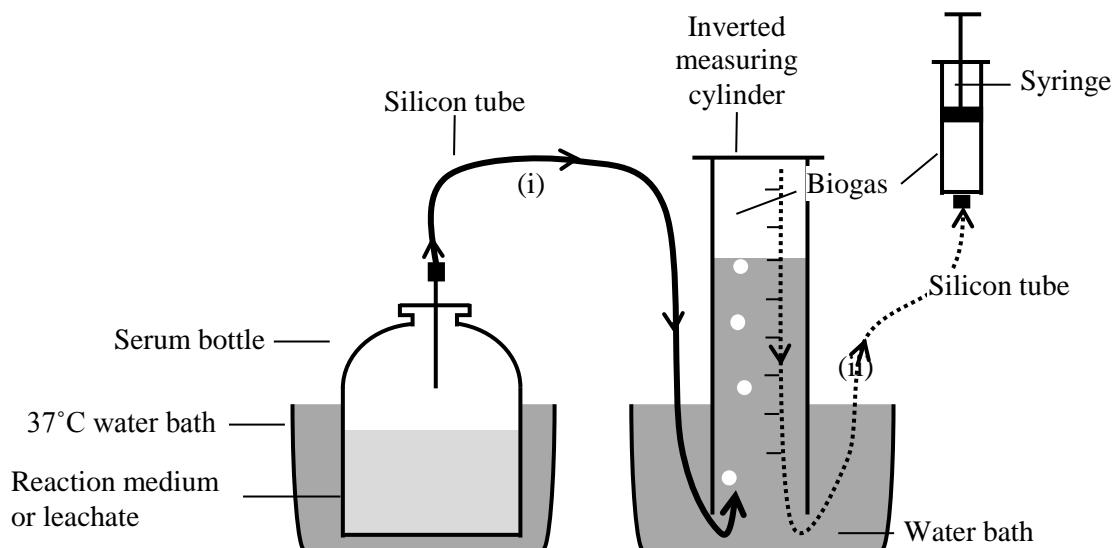
Figure 3.2: Experimental setup of batch mode dark fermentation. Direction (i): the collection of biogas flow from serum bottle to measuring cylinder; direction (ii): the collection of biogas from measuring cylinder to syringe. Silicon tube and syringe were flushed with argon gas.
