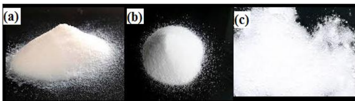
Figure 3.4: Image of a) HDTMS nano-silica, b) DDS nano-silica and c) HMDZ nano-silica
