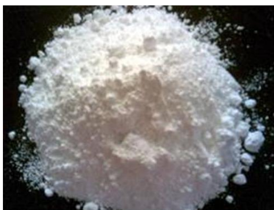
Figure 3.3: Nano-ZnO powder (size 20-30 nm) used in present work
