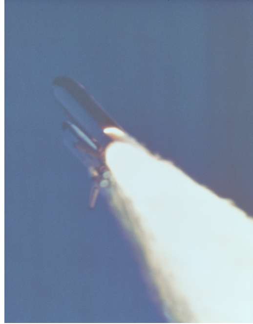
(b) Plume of exhaust leaking from Challenger's left booster. ©NASA, http://grin.hq.nasa.gov/ABSTRACTS/GPN-2000-001425.html
