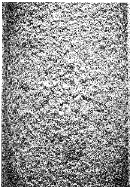
Fig. 5. As-sprayed \text{ZrO}_2 -8wt.% \text{Y}_2\text{O}_3 specimen after 15 cycles of 2.5 s (case B) in a 30 kW plasma flame.
