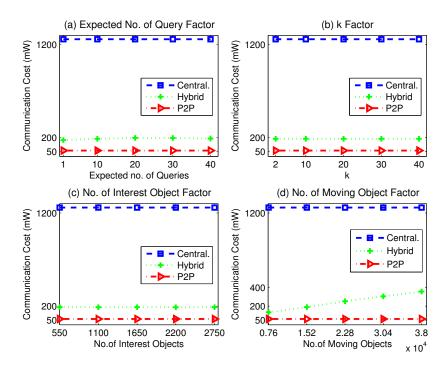
Figure 6.5: Communication Cost among Centralized, Hybrid and P2P Systems
