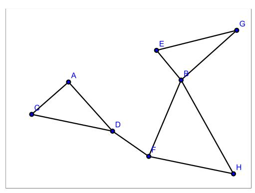
Figure 2.14: An illustration of a All-2NN query. A line is drawn between two objects if one object is one of two nearest neighbours of another.
