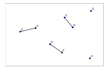
Figure 2.16: An illustration of an Reflexive-1NN query. A line is drawn between two objects if they are nearest neighbours of each other.
