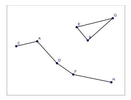
Figure 2.17: An illustration of a Reflexive-2NN query. A line is draw between two objects if one object is one of 2 nearest neighbours of another and vice versa.
