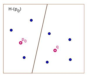
Figure 2.18: Half-space pruning. Any point that lies in the shaded half- space  $H^{-}(p_0)$  is always closer to  $p_0$  than to q and cannot be the RNN for this reason.
