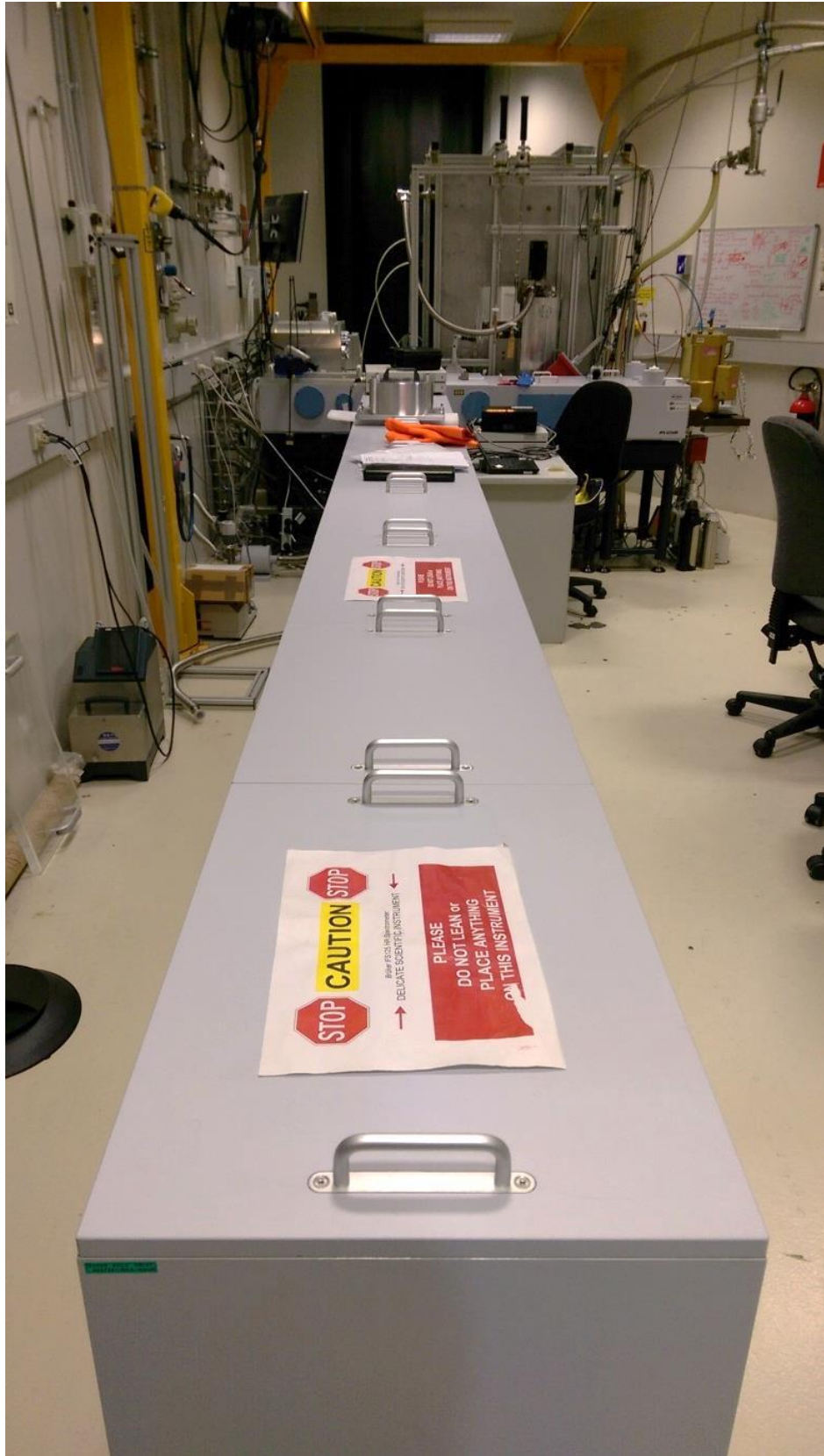
Figure 1.6: The Bruker IFS125 HR Spectrometer at the Australian Synchrotron THz/far-IR beamline. Pictured is the interferometer arm, with the enclosive flow cooling (EFC) cell manifold in the background
