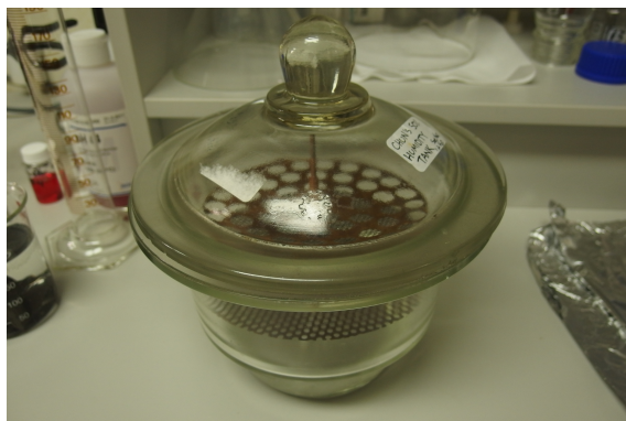
Figure 2.2: The humidity chamber with saturated NaCl solution and constant humidity at 75%
