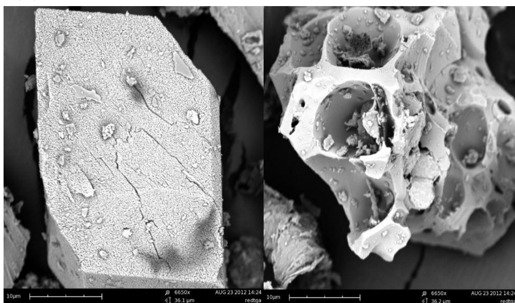
Figure 8.2.3 Structure of commercial wood mix (less than 38 μm) - (a) raw (b) char obtained from TGA.
