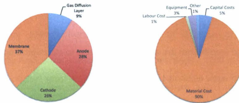
Figure 1.3: (a) Membrane Electrode Assembly Cost Breakdown for 2001 System Configuration 11 , (b) Membrane Cost Breakdown 11
