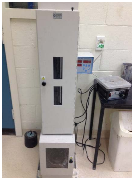
Figure 3-4: An automatic compaction machine
