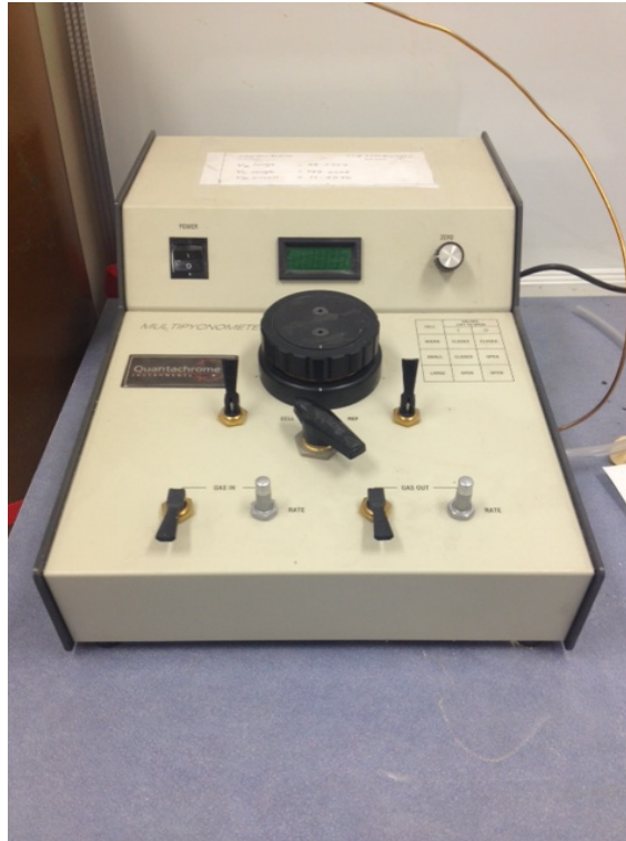
Figure 3-3: Multipycnometer. An automatic soil specific gravity testing instrument
