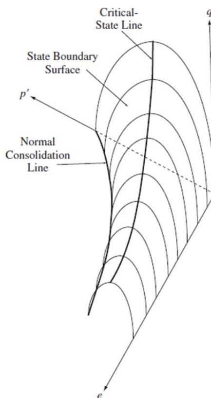
Figure A.4 State boundary surface of the Cam-clay model (Helwany, 2007)
