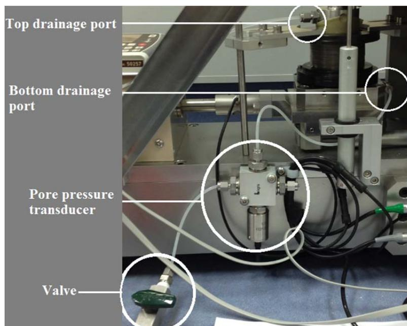
Figure 3.7 Pore pressure measurement configuration
