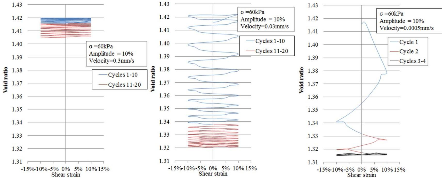
Figure 4.12 Void ratio versus shear strain plots for applied vertical stress of 60kPa and shear amplitude of 10% of H
