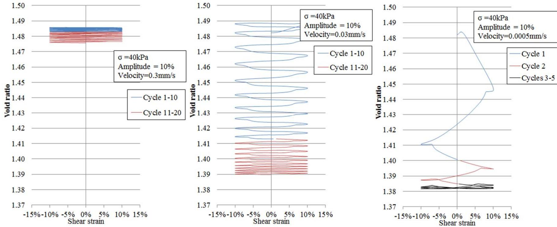
Figure A.8 Void ratio versus shear strain plots for applied vertical stress of 40kPa and shear amplitude of 10% of H
