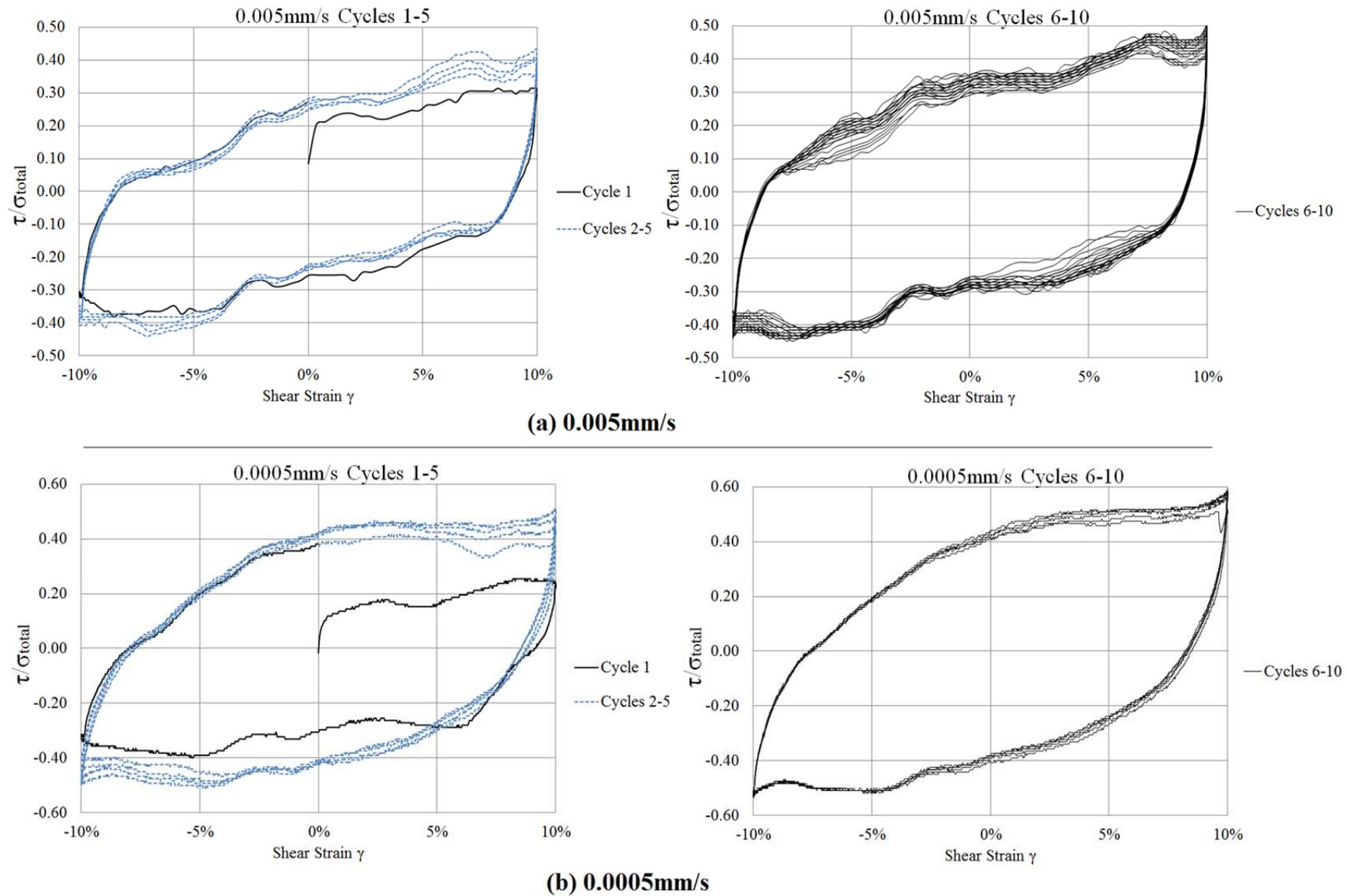
Figure 3.17 Shear stress-strain relationship for (a) 0.005mm/s and (b) 0.0005mm/s
