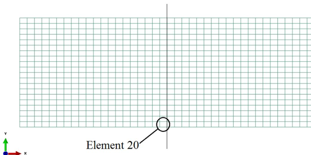
Figure 4.5 Excess pore pressure reference element
