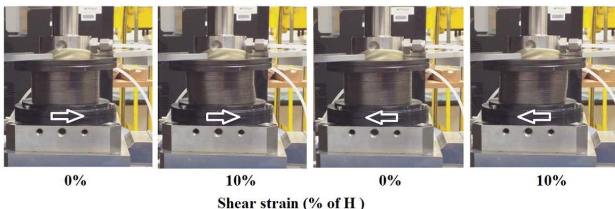
Figure 3.13 Cyclic shearing of the soil specimen
