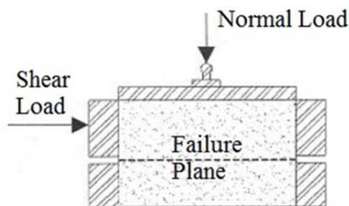
Figure 2.12 An illustration of the direct shear box (Zekkos et al., 2010)
