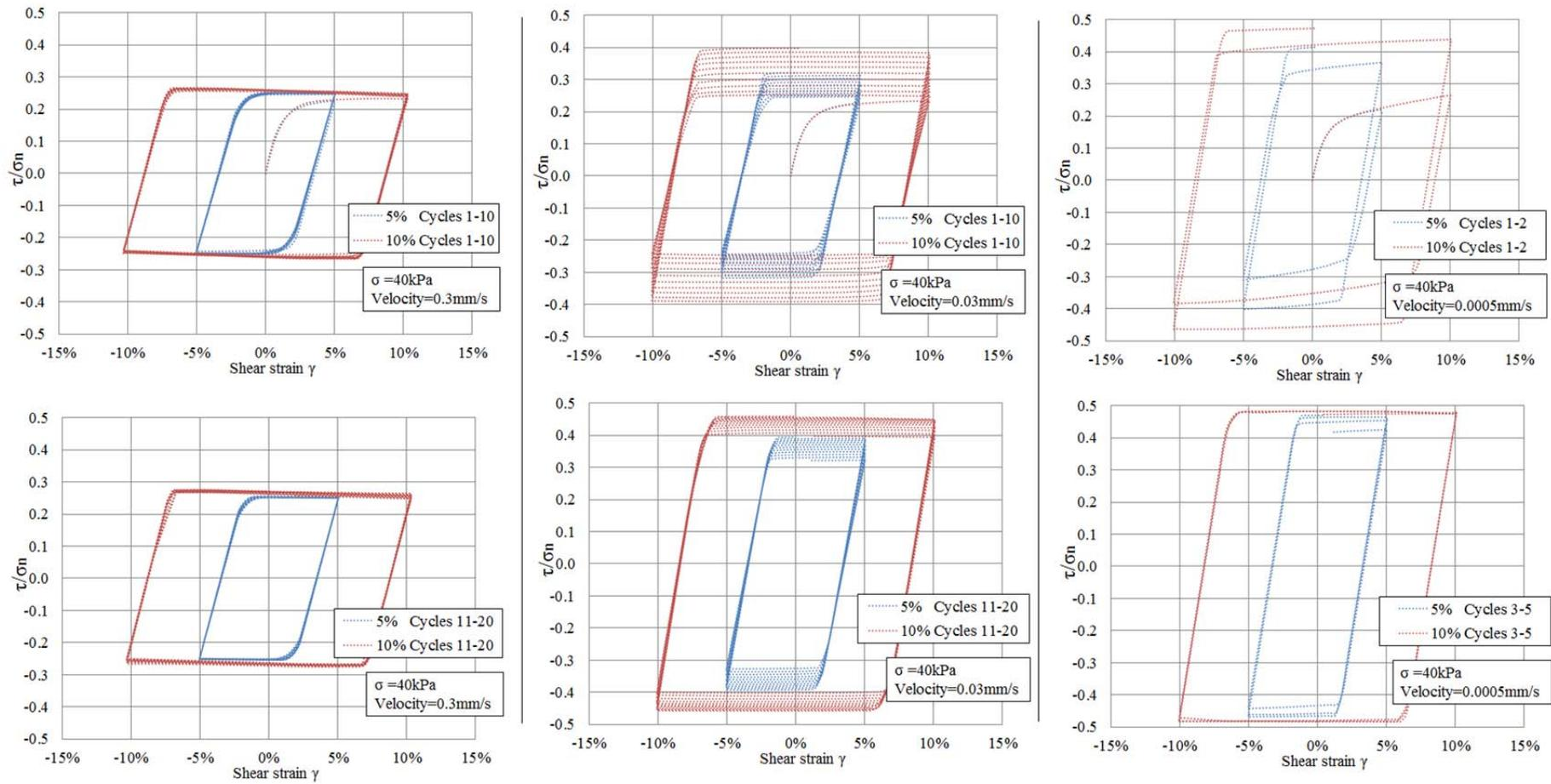
Figure A.10 Shear stress-strain curves for applied vertical stress of 40kPa
