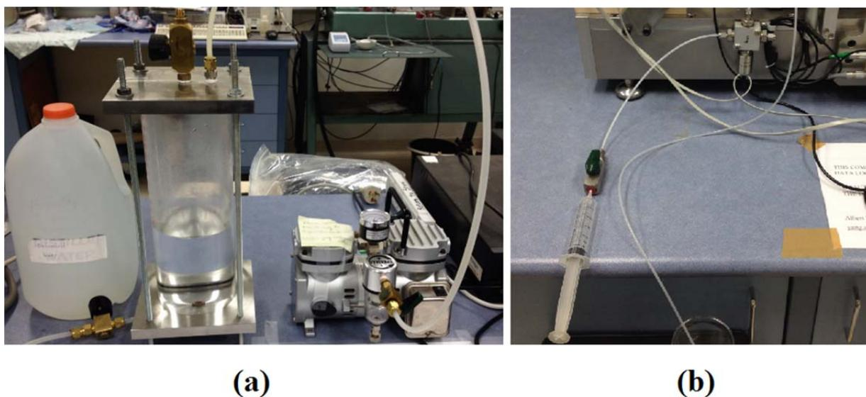
Figure 3.8 (a) De-airing water apparatus (b) Water injection
