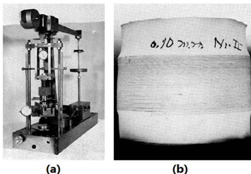
Figure 2.15 (a) NGI direct simple shear device (b) Reinforced rubber membrane (Bjerrum and Landva, 1966)
