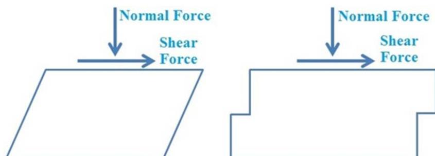
Figure 2.13 Illustrations of direct simple shear test (left) and direct shear test (right)
