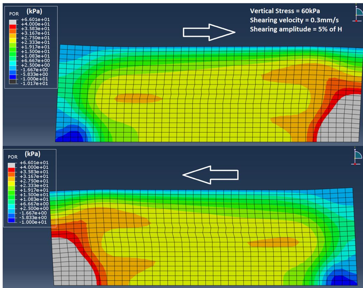
Figure 4.8 Pore pressure distribution at cyclic shearing stage
