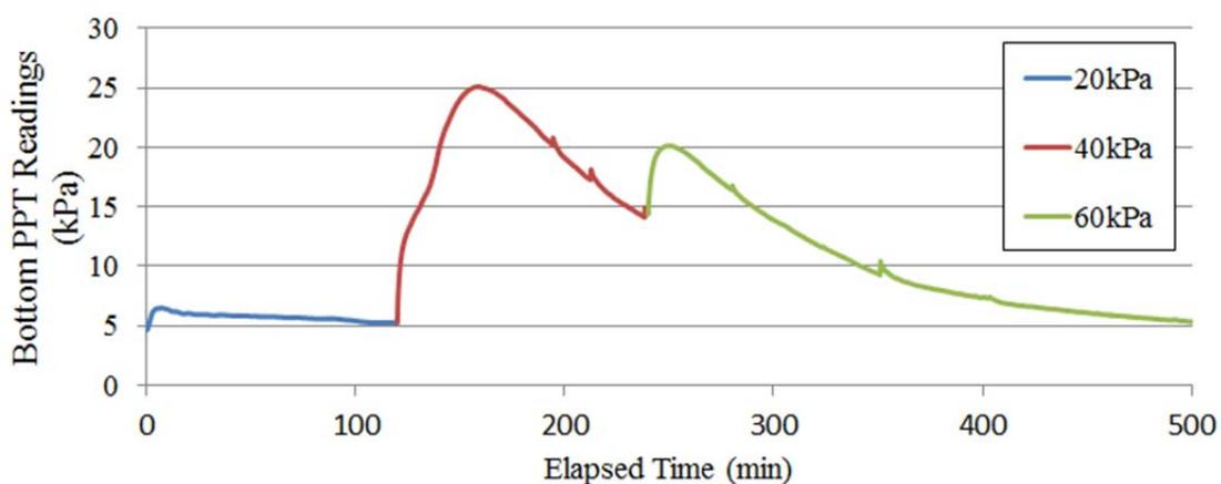
Figure 3.12 PPT Readings at consolidation stage
