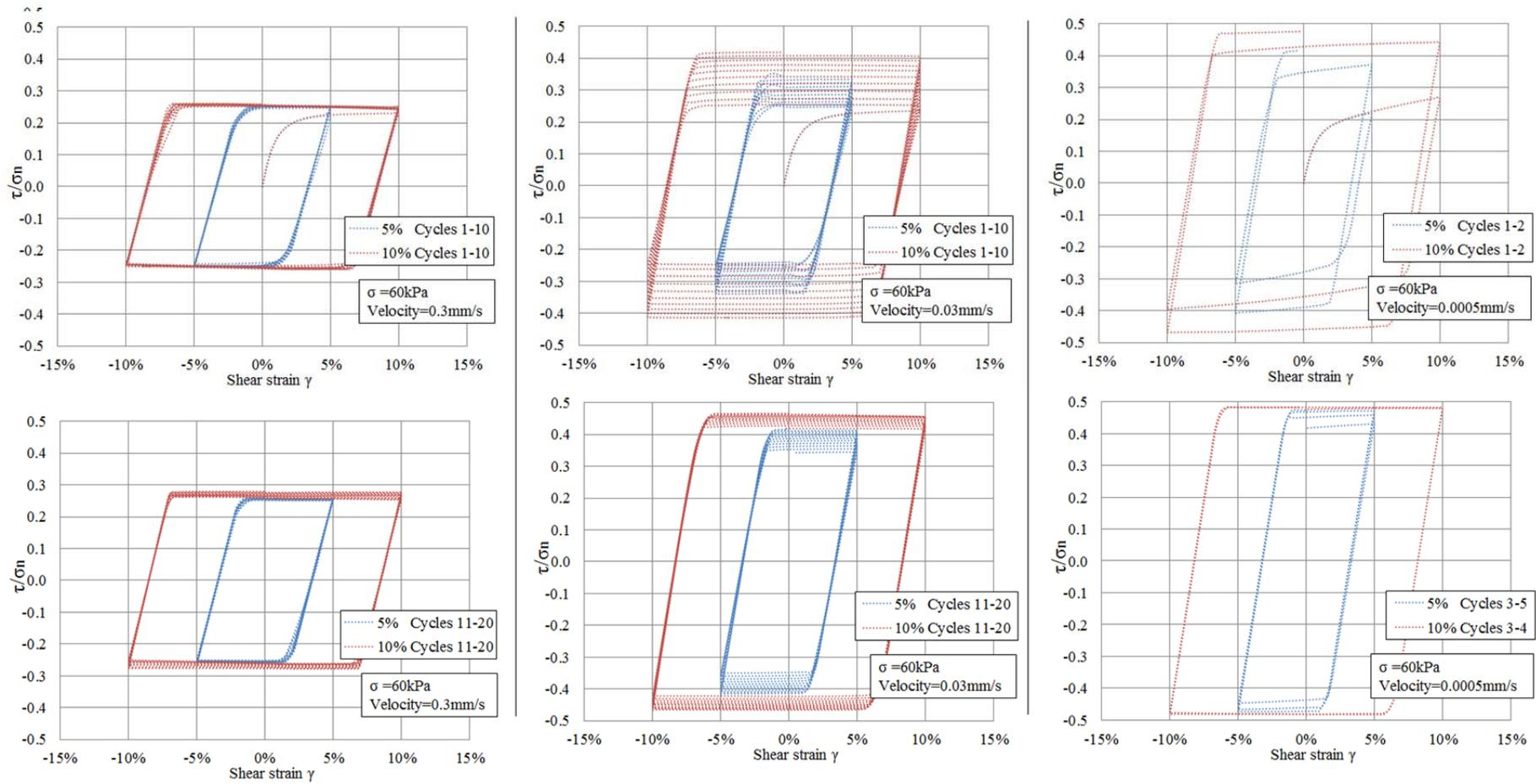
Figure 4.14 Shear stress-strain curves for applied vertical stress of 60kPa
