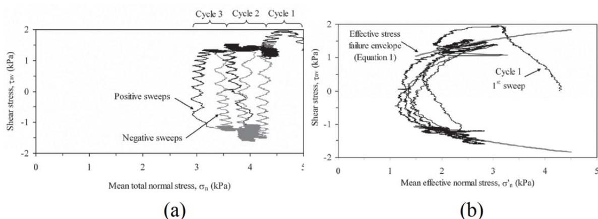
Figure 2.5 (a) Total stress interpretation of axial response (b) Effective stress interpretation of axial response (White et al., 2011b)
