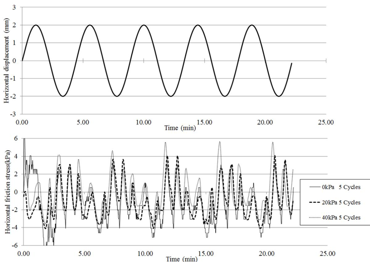
Figure 3.10 Variations in horizontal load readings due to rail friction
