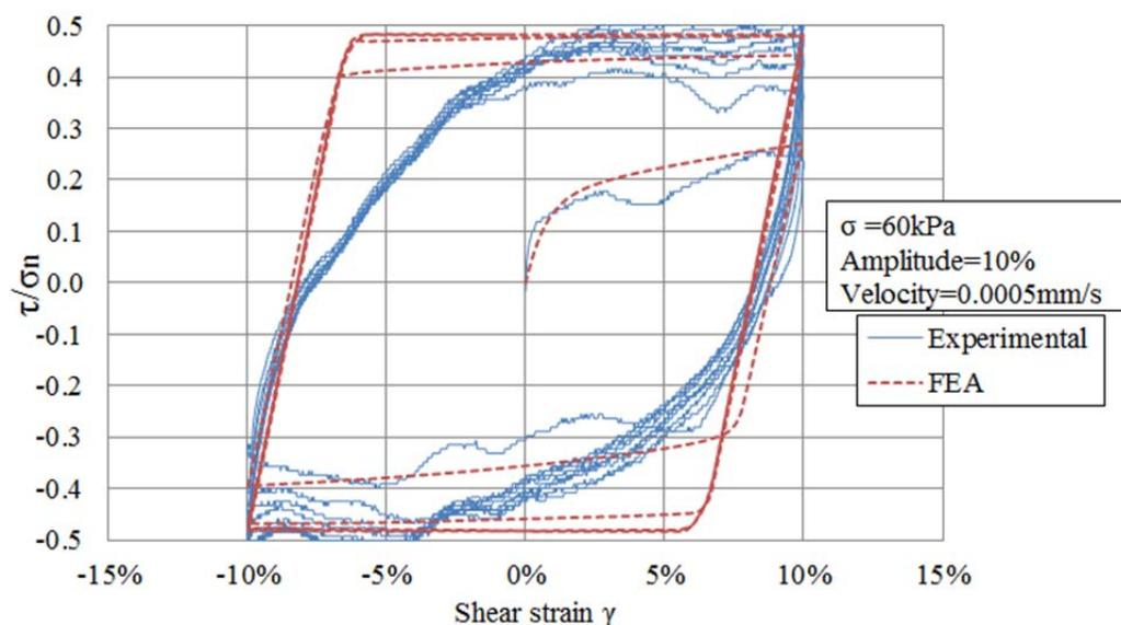
Figure 4.3 Comparison between experimental and FEA shear stress-strain curves
