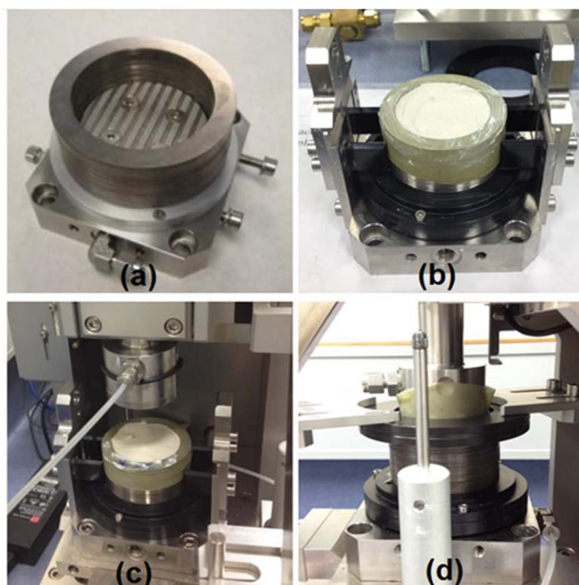
Figure 3.6 Specimen preparation and insertion
