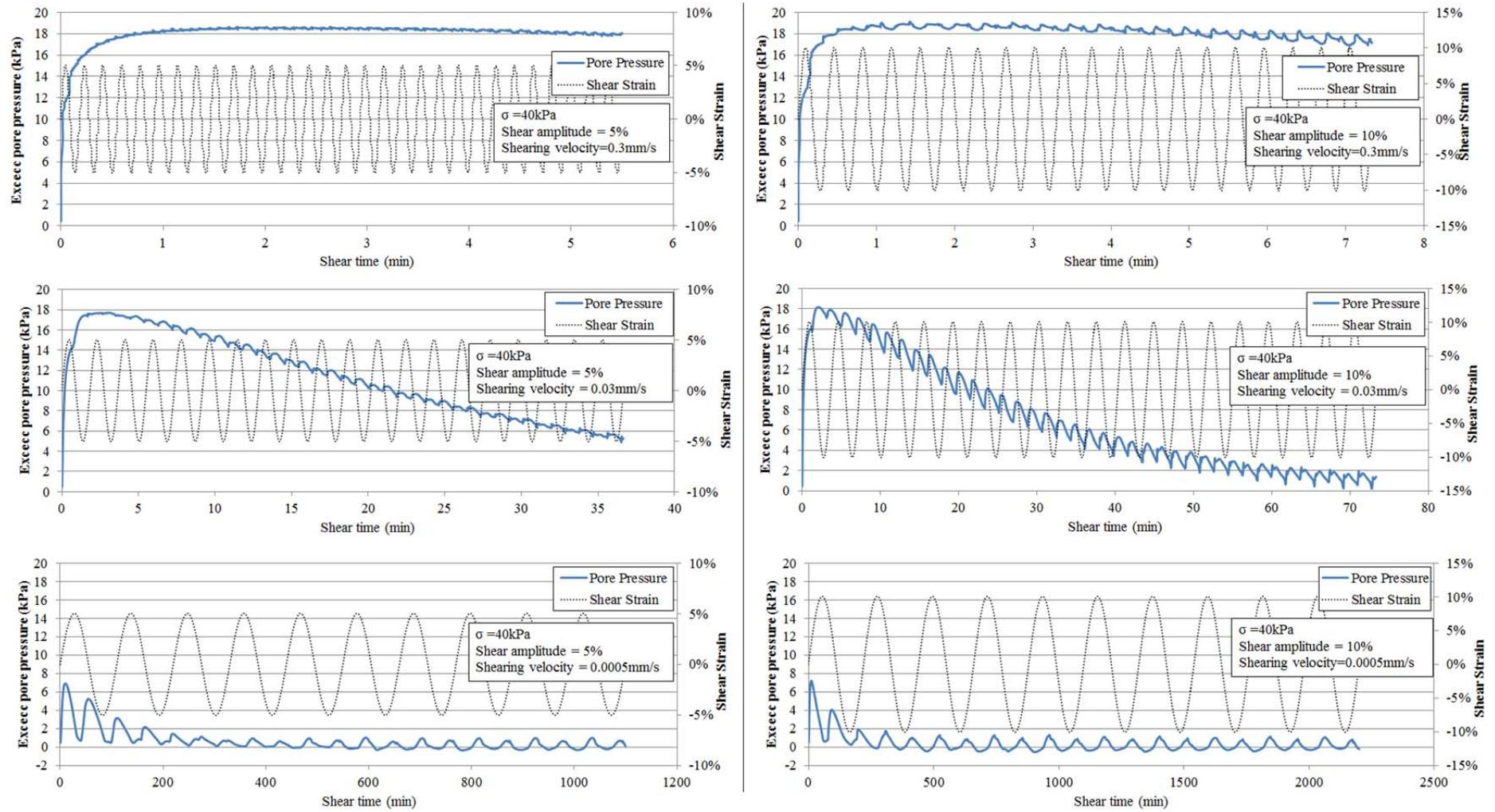
Figure A.6 Excess pore pressure development at cyclic shearing stage for applied vertical stress of 40kPa
