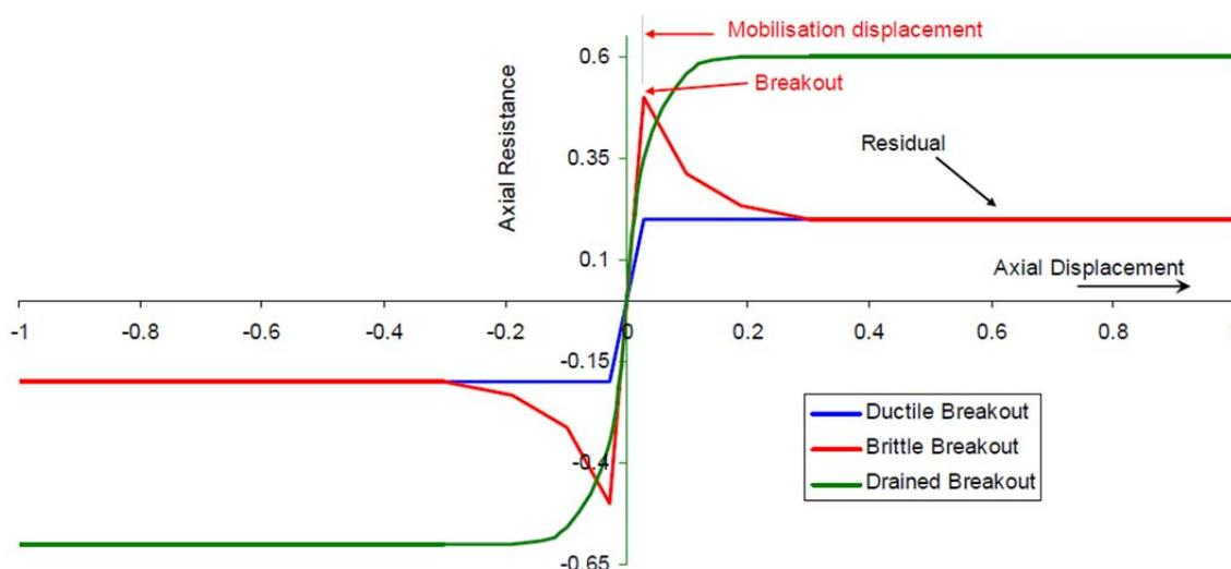
Figure 2.1 Axial friction resistance schematic with mobilisation displacement and breakout (Bruton et al., 2008)
