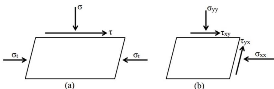
Figure 2.16 Stresses acting on test sample: (a) in direct simple shear apparatus; (b) in true simple shear (Airey and Wood, 1987)
