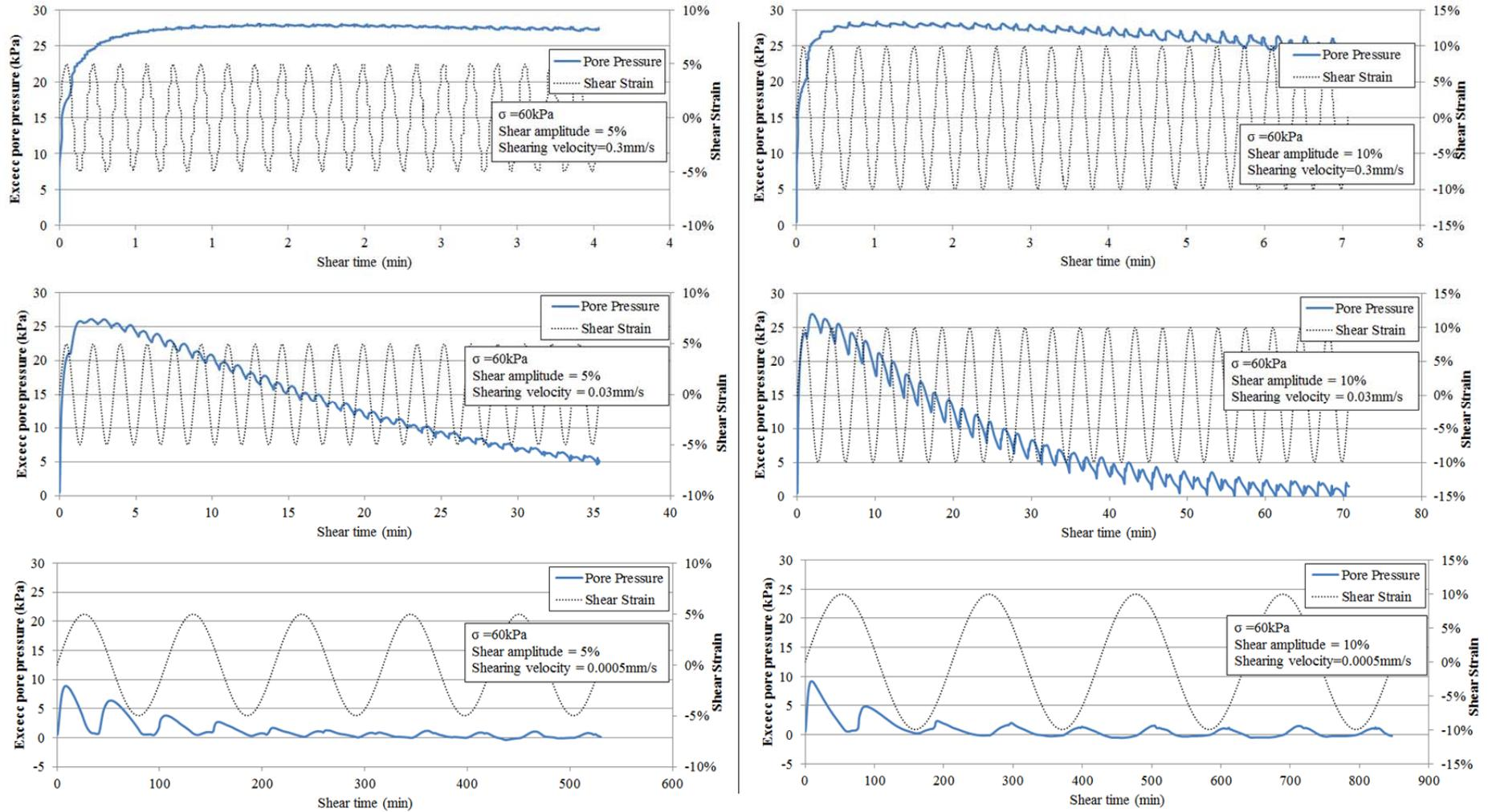
Figure 4.10 Excess pore pressure development at cyclic shearing stage for applied vertical stress of 60kPa
