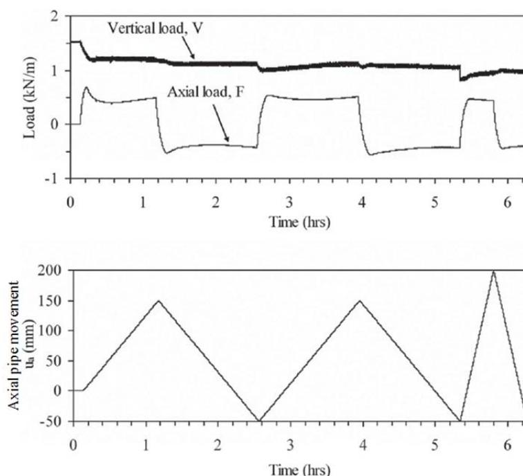
Figure 2.3 Time history during cyclic axial pipe testing (White et al., 2011b)
