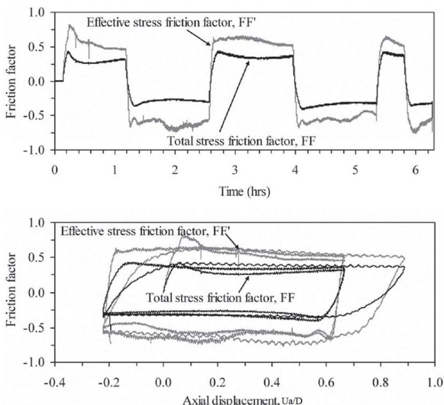
Figure 2.4 Friction factor response in cyclic axial pipe testing (White et al., 2011b)
