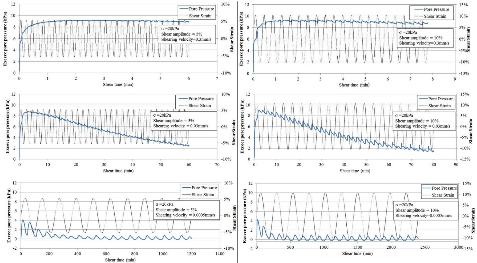
Figure A.5 Excess pore pressure development at cyclic shearing stage for applied vertical stress of 20kPa
