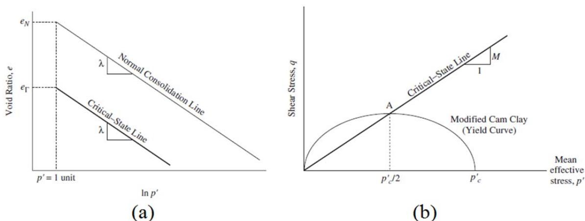
Figure A.3 (a) Normal consolidation and critical state lines in the  $e$ - $\ln p'$  plane (b) yield surface of a Cam-clay model in the  $q$ - $p'$  plane (Helwany, 2007)
