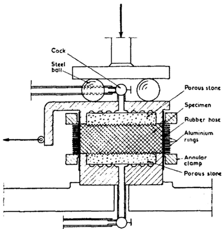
Figure 2.14 S.G.I Direct Simple Shear Device (Kjellman, 1951)
