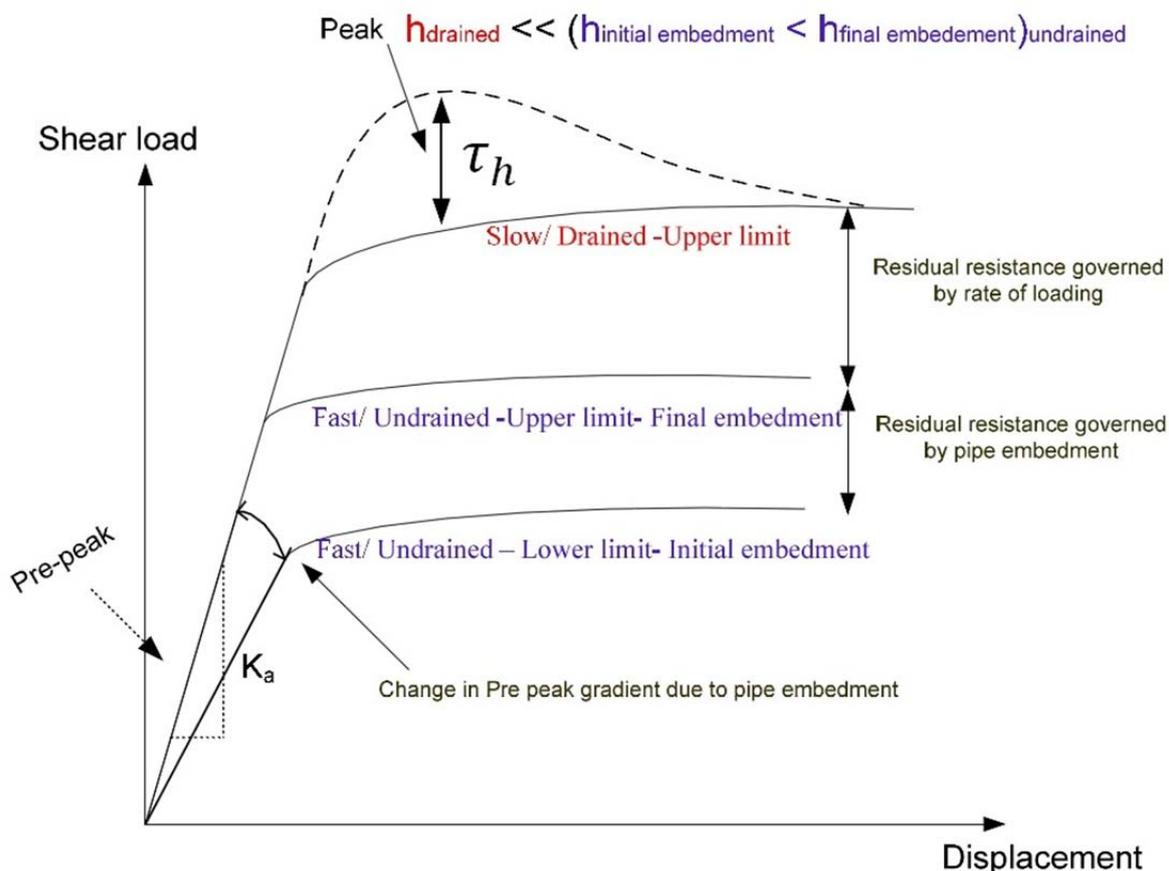
Figure 2.10 Generic pipe load-displacement curve with emphasis on residual resistance (Senthilkumar, 2013)
