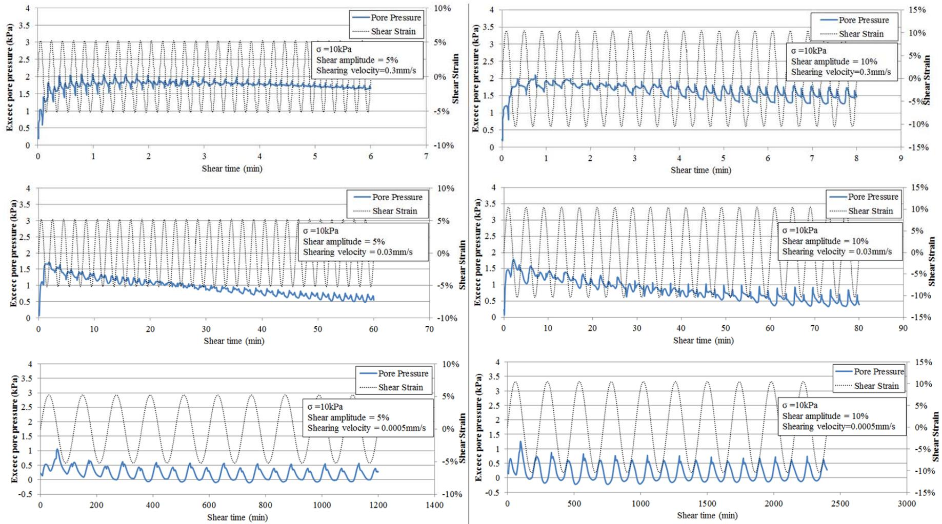
Figure 4.9 Excess pore pressure development at cyclic shearing stage for applied vertical stress of 10kPa
