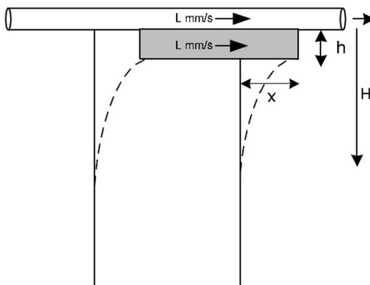
Figure 2.8 Shear zone underneath axially-walking pipe (Senthilkumar, 2013)
