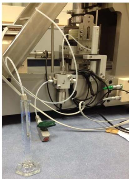
Figure 3.9 Measuring cylinder connecting to the top drainage port
