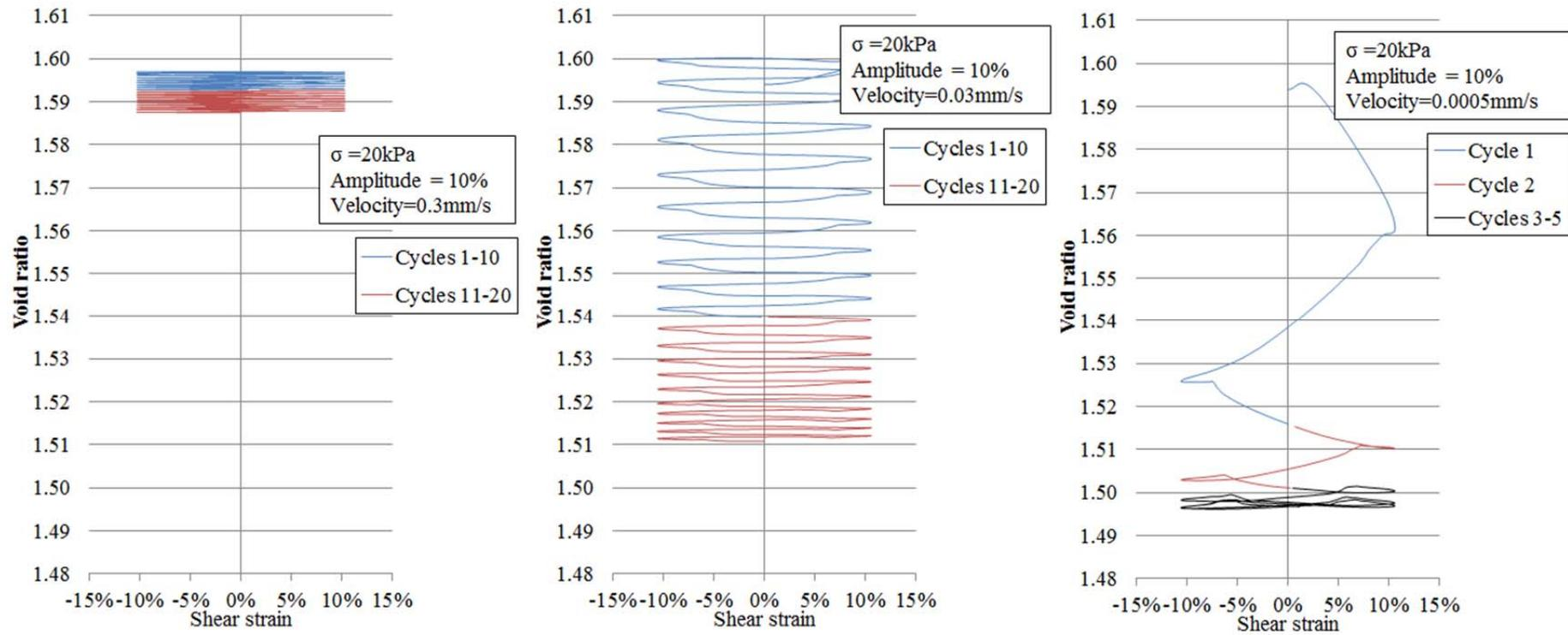
Figure A.7 Void ratio versus shear strain plots for applied vertical stress of 20kPa and shear amplitude of 10% of H
