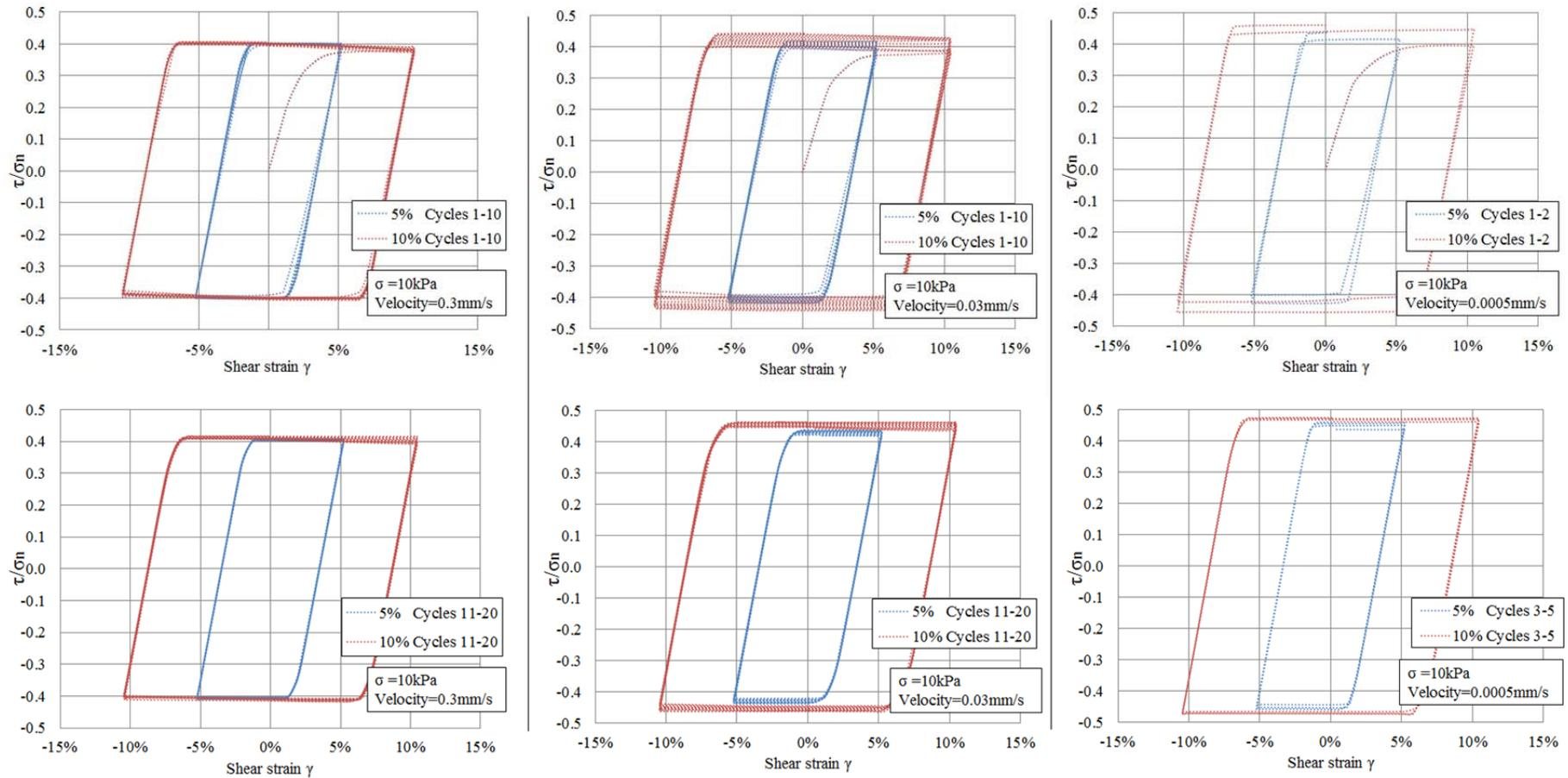
Figure 4.13 Shear stress-strain curves for applied vertical stress of 10kPa
