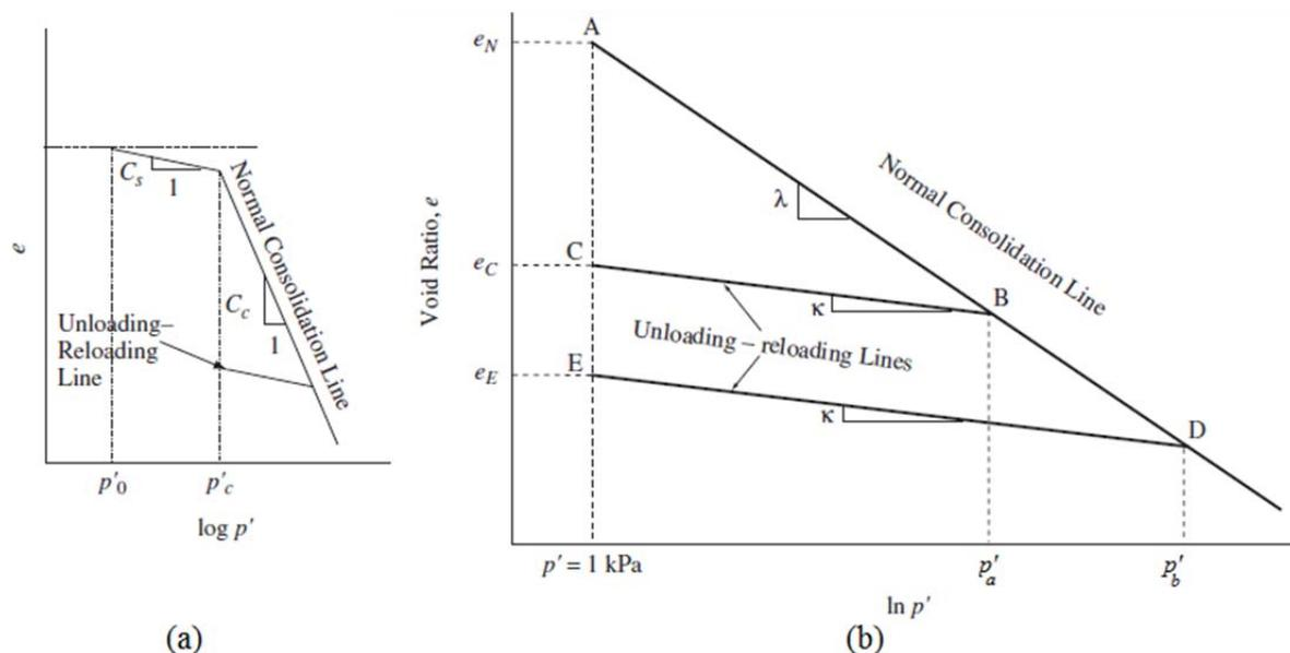
Figure A.1 (a)  $e$ - $\log p'$  curve of an isotropic consolidation test and (b) consolidation curve in the  $e$ - $\ln p'$  plane (Helwany, 2007)
