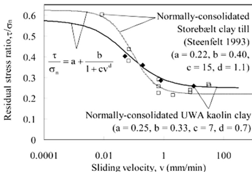
Figure 2.2 Interface shearing: kaolin clay and Storeælt clay till (White and Cathie, 2011, Steenfelt, 1993)
