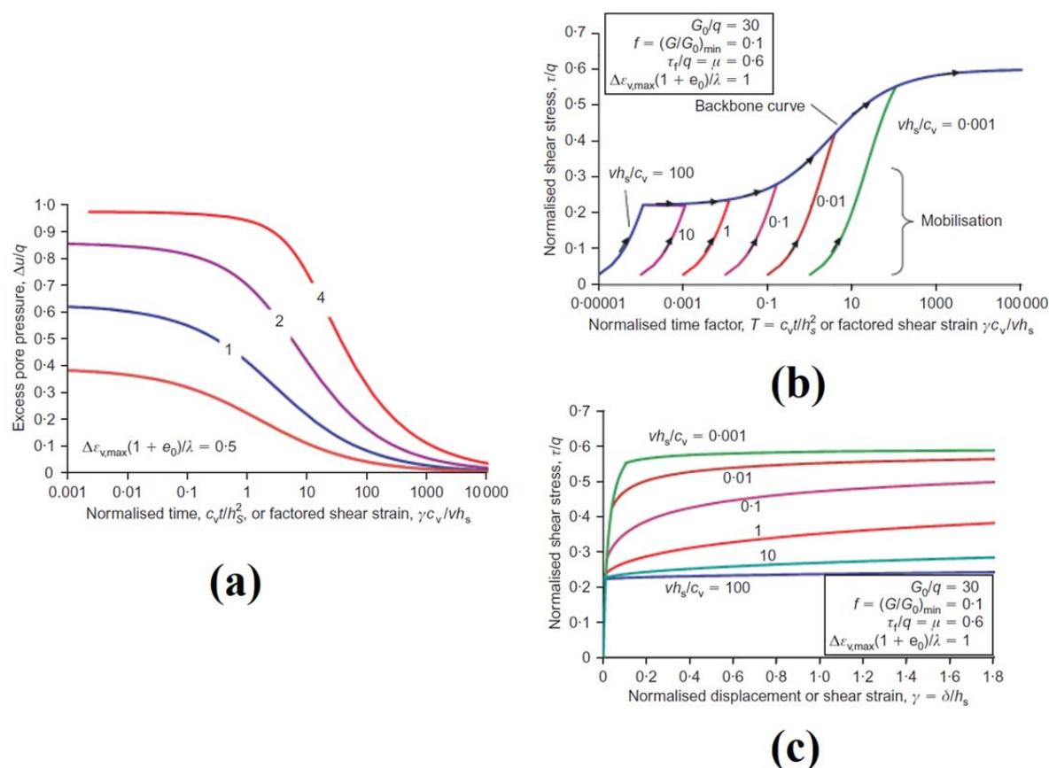
Figure 2.7 (a) Example relationships between excess pore pressure and time or shear strain Planar shearing responses for different normalised velocities Variation in resistance with (b)time; (c)displacement (Randolph et al., 2012)
