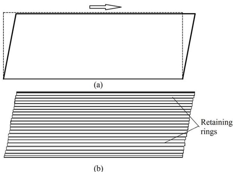
Figure 4.2 Implementation of deformation pattern in cyclic shearing in FEA model
