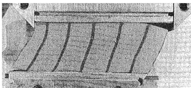
Figure 2.17 Side view of a plasticine sample after shearing under a normal stress of 12kPa (Roscoe, 1953)
