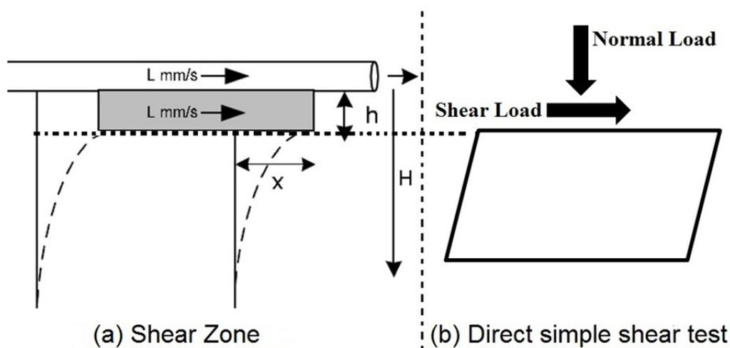
Figure 2.9 (a) Shear zone underneath axially walking pipe and (b) loading pattern of direct simple shear test
