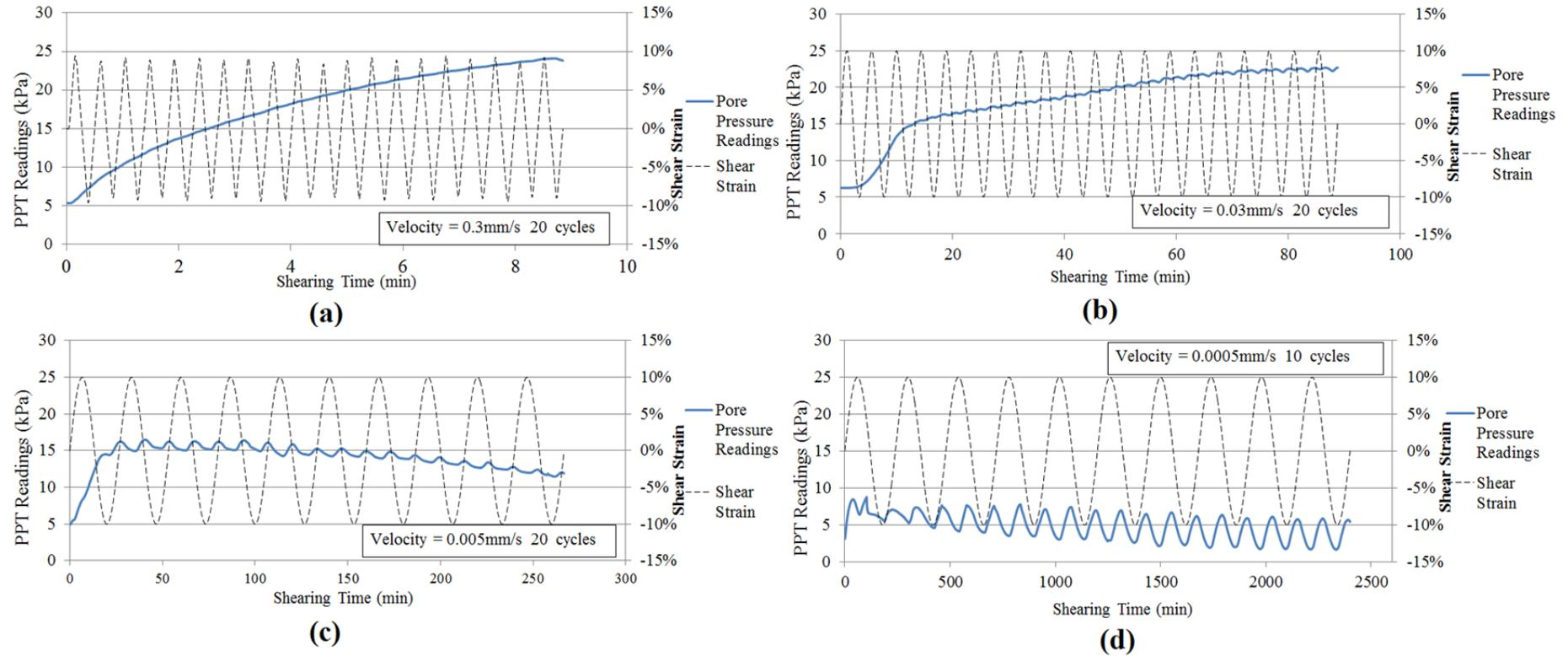
Figure 3.14 Excess pore pressure development at shearing stage
