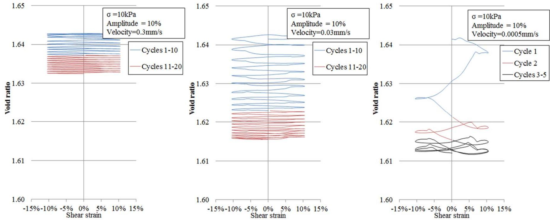
Figure 4.11 Void ratio versus shear strain plots for applied vertical stress of 10kPa and shear amplitude of 10% of H
