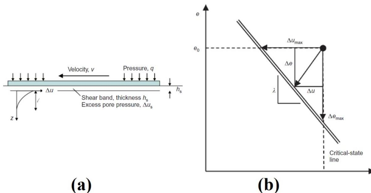
Figure 2.6 (a) Schematic diagram for analysis of velocity effects for planar shearing (b) Stress paths in  $e-\ln\sigma_v$  space (Randolph et al., 2012)
