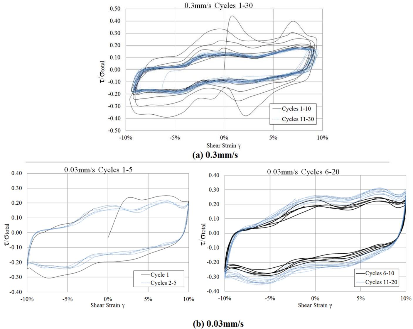
Figure 3.16 Shear stress-strain relationship for (a) 0.3mm/s and (b) 0.03mm/s
