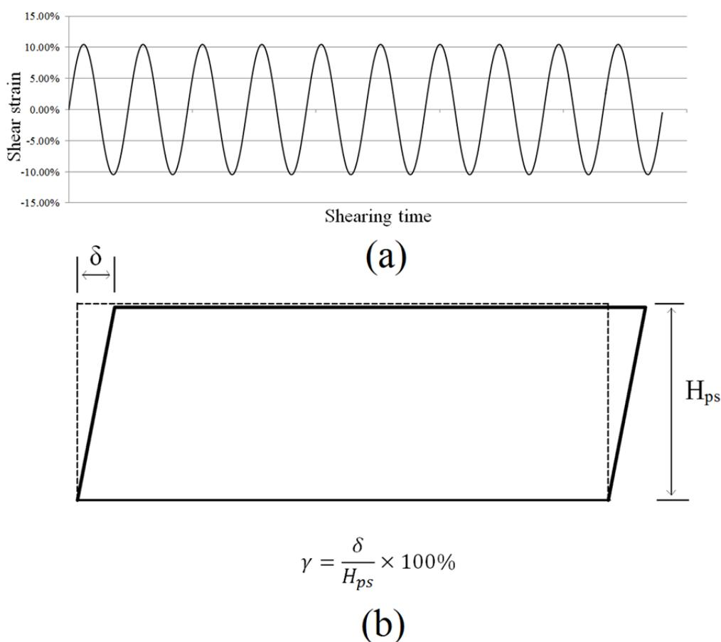
Figure 4.7 (a) horizontal displacement function and (b) shear strain definition
