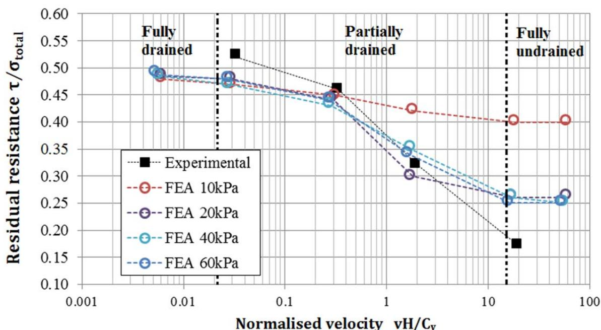
Figure 4.16 Residual resistance versus normalised velocity
