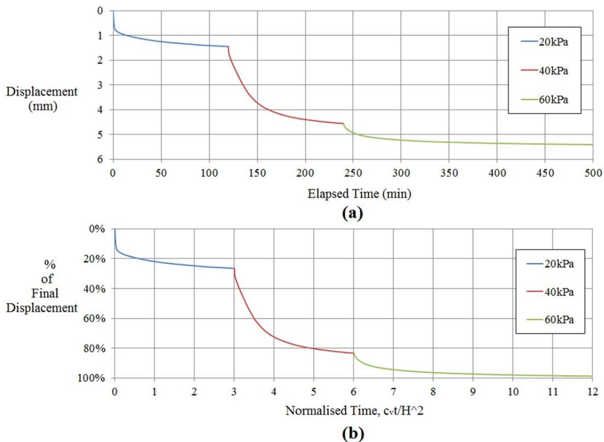
Figure 3.11 Consolidation displacement vs. (a) Elapsed time (b) Normalised time
