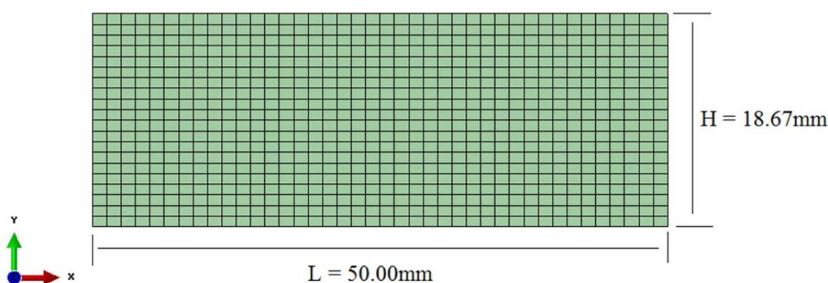
Figure 4.1 Two-dimensional finite element model
