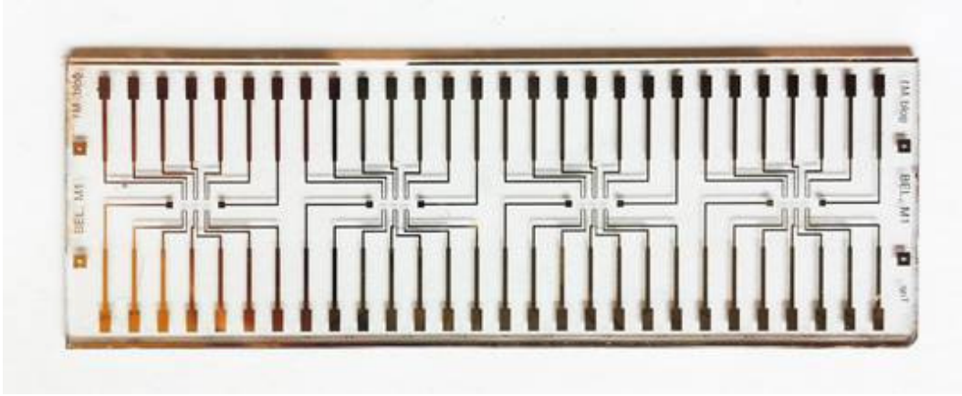
Figure S4 Array of PEDOT:PSS channels with gold connectors on glass substrate. The patterning was made via photolithography techniques.
