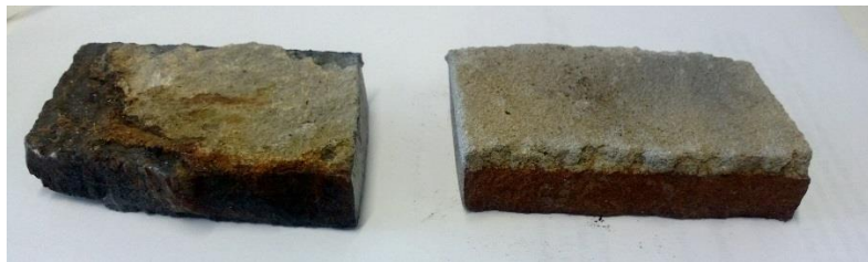
Figure 7- 18 Specimens from fracture surface: dark grey colour (left) and orange-brown (right)
