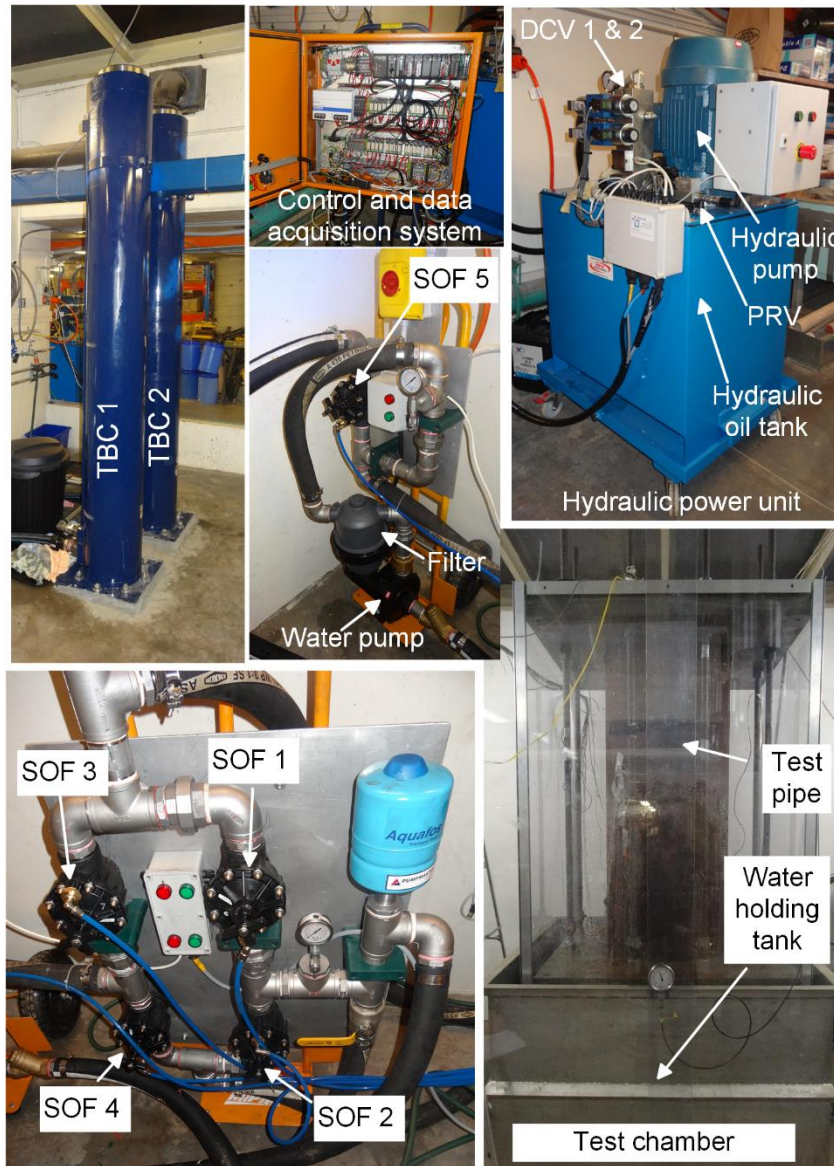
Figure 7- 3 Components of pipe fatigue test facility
