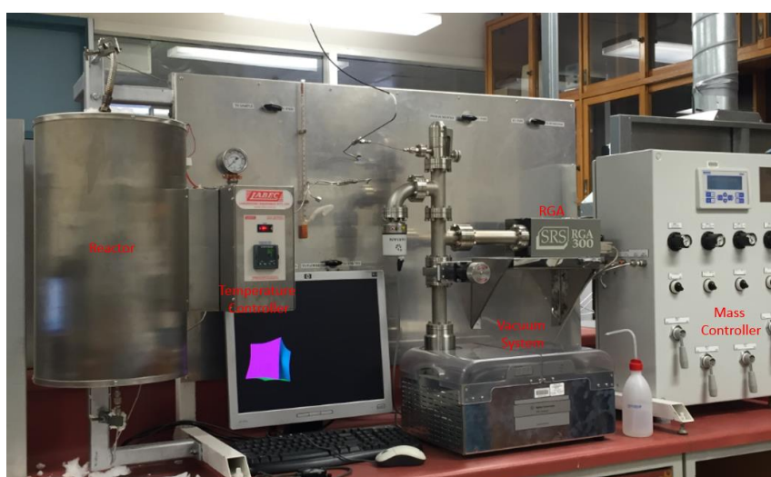
Figure 3.3.4-1: CO-Temperature Programmed Desorption set up
