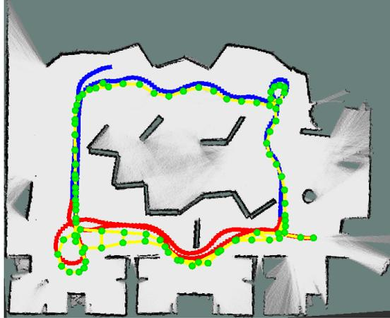
**Figure 3.9:** Reference graph map for odometry correction cost comparison. The robot started performing SLAM from the bottom right corner of the map on Carpet 1. Then it was steered clock-wise on Carpet 1 and Blue Rubber, on which the trajectories were shown as red and blue lines, respectively. Green dots represent robot positions and yellow lines represent relative robot poses. Reused from [1] ©2015 IEEE.
