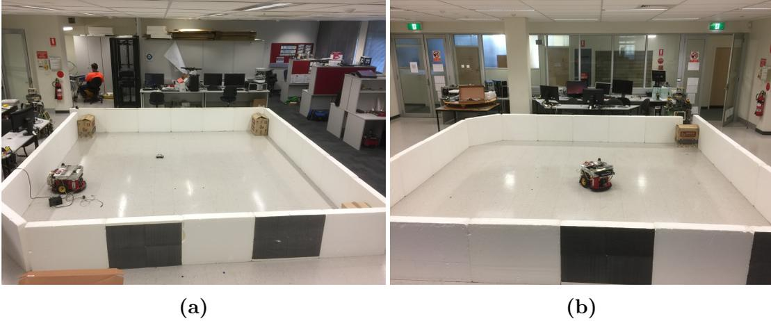
**Figure B.2:** The testing environment for measuring the robot slip angles on circular paths on Lino. (a) Robot is being charged. (b) Robot is automatically driving in a circle.
