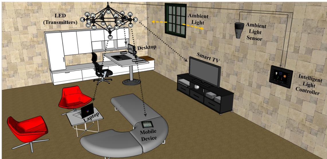
Figure 3.26: Concept of VLC system integrated with an intelligent lighting framework
