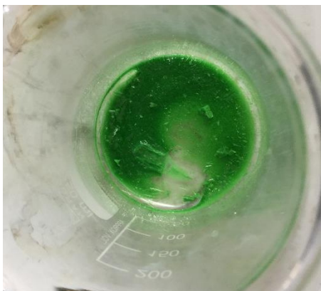
Figure 3.4: Xerogel of nickel oxide precursor
