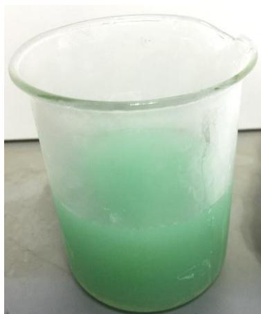
Figure 3.3: Sol solution of nickel acetate-gelatin
