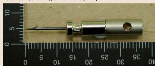
Taser dart, showing dimensions (mm)
