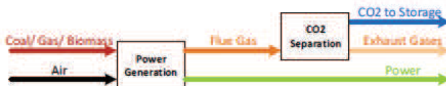
Figure 1: Membrane and Low-Temperature Hybrid Carbon Capture Schematic Diagram
