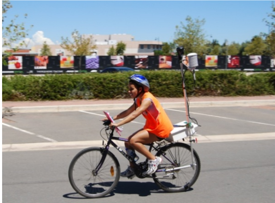
Figure 3.11: A photograph of the setup of the instrumentation on the back of a bicycle. This setup was used for data collection during the transect data collection.
