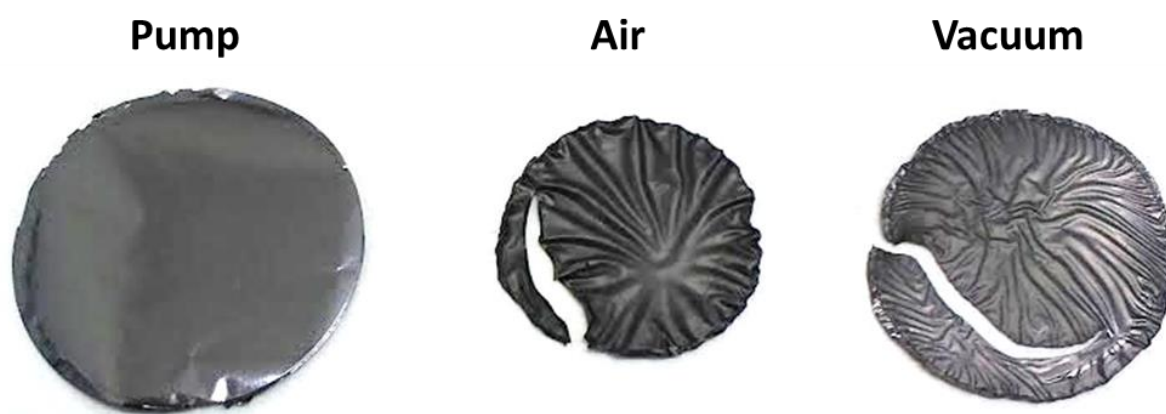
Figure 46. Comparison of rGO assemblies that were pump dried, air dried, or vacuum dried, showing the tendency of the material to shrink under different conditions. All assemblies shown here have the same mass.
