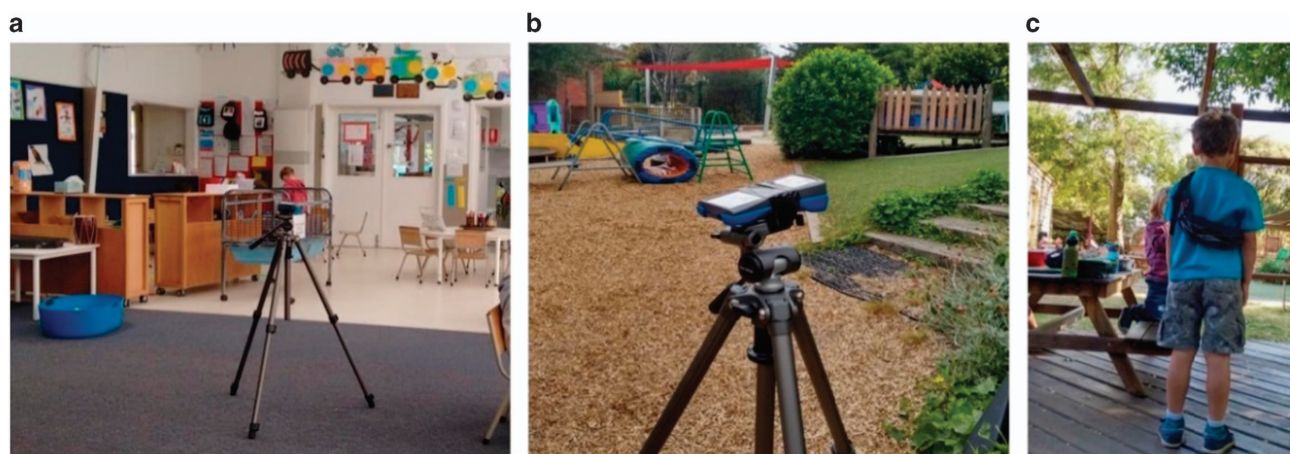
Figure 2. Measurement setups: an indoor (a), outdoor (b) (environmental) and personal (c) exposure measurements in a kindergarten (pictures taken with the permission of the kindergarten directors).
