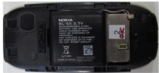
Fig. 2 The rear view of a hardware modified phone (the battery is wired to special hardware inside the handset)
