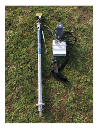
FIGURE 4.2. Soil respiration, soil temperature, and soil moisture equipment used in both plantation and pasture.
