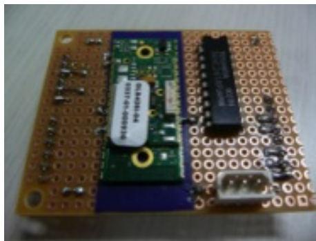
Figure A.21: Finished soldered shield board.
