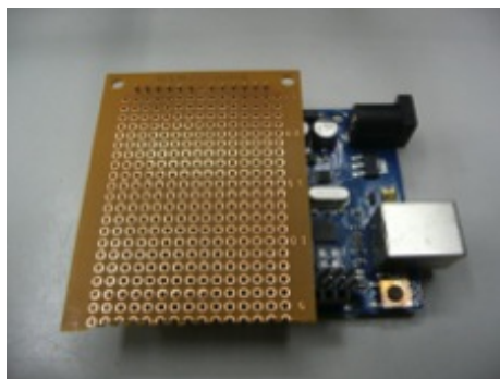
Figure A.15: Preparing the soldering pin socket to the universal board as Arduino shield.
