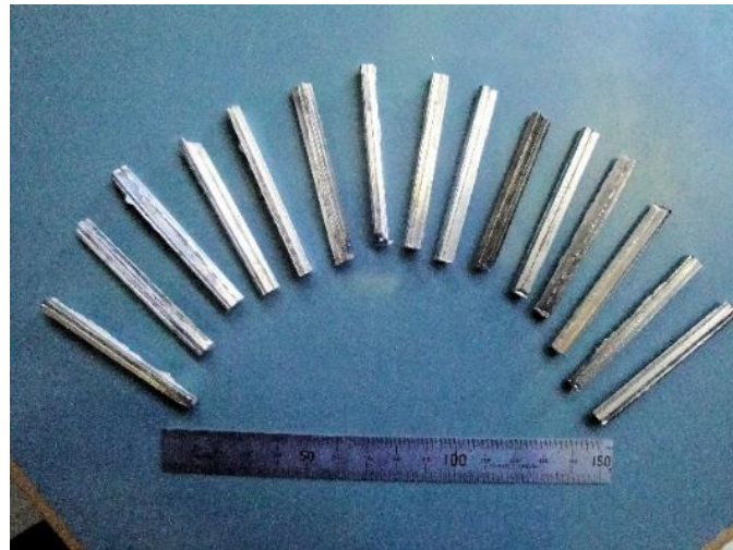
Figure 25 Rotocast \text{Mg}_{60}\text{Cu}_{29}\text{Gd}_{11} bars.
