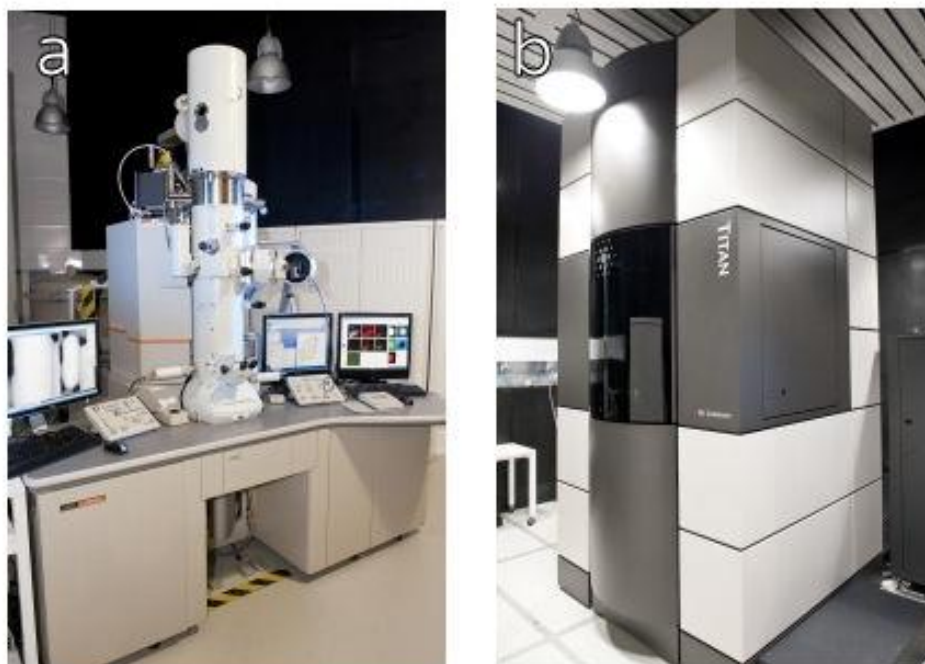
Figure 21 (a) JEOL JEM-2100F FEGTEM. (b) Double-corrected FEI Titan 3 80-300 FEGTEM.
