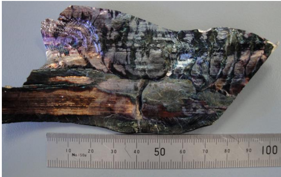
Figure 36 Strip produced from \text{Mg}_{60}\text{Cu}_{29}\text{Gd}_{11} at high casting speed. The strip surface is multicoloured which is an indication of oxidation.
