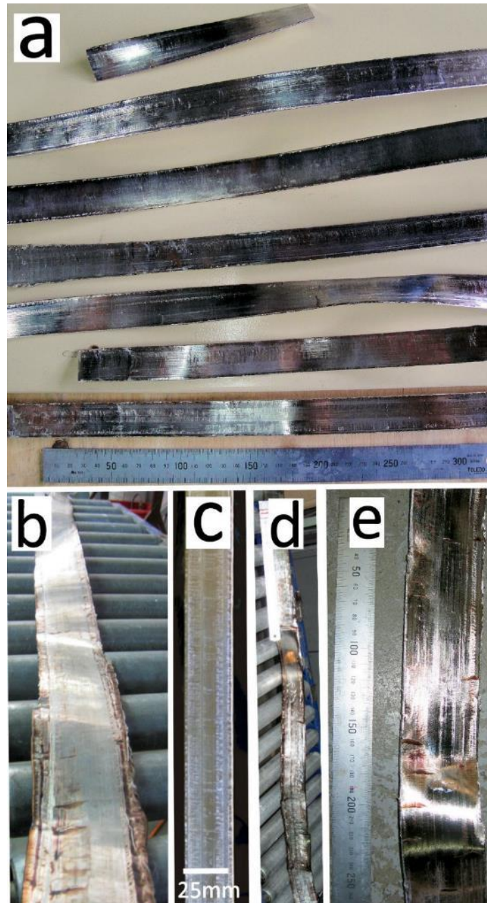
Figure 34 Sheet material produced by TRC from various casting experiments. (a) \text{Mg}_{66}\text{Cu}_{25}\text{Y}_9 sheet 1 mm thick produced from one cast run. (b) \text{Mg}_{60}\text{Cu}_{29}\text{Gd}_{11} sheet 2 mm thick 75 mm wide. (c) \text{Mg}_{66}\text{Cu}_{25}\text{Y}_9 sheet 1 mm thick surface detail. (d) \text{Mg}_{60}\text{Cu}_{29}\text{Gd}_{11} sheet 2 mm thick 75 mm wide. (e) 3 mm thick \text{Mg}_{60}\text{Cu}_{29}\text{Gd}_{11} sheet 50 mm wide.
