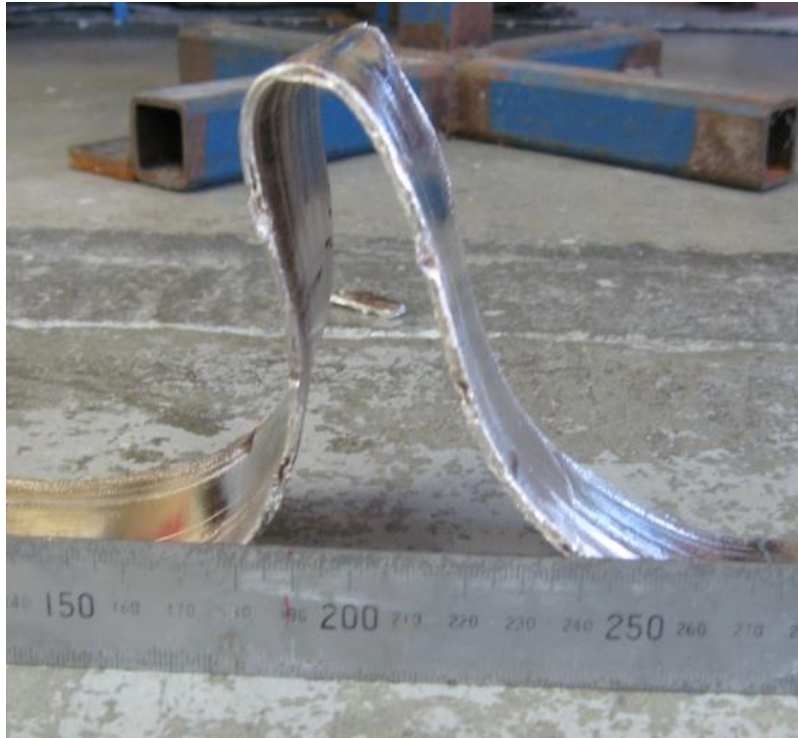
Figure 43 As-cast twin roll cast sheet of \text{Mg}_{60}\text{Cu}_{29}\text{Gd}_{11} . This section is unsupported on the run out table causing a large bend in strip. The tensile stress in the outer surface can cause hot tear defects.
