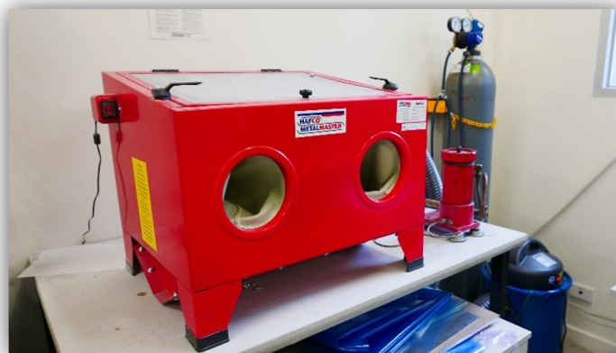
Figure 3.17 Grit blasting machine used to surface prep adherend surfaces for bonding
