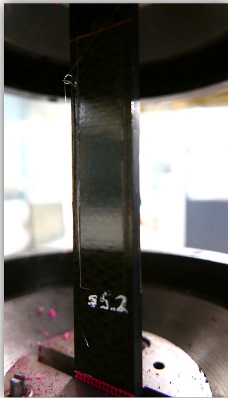
Figure 6.9 Fibre optic cable bonded to one face of Configuration 2.5
