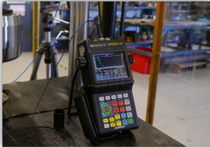
Figure 2.18 Non-destructive testing using an Olympus Epoch XT ultrasonic A-scanner
