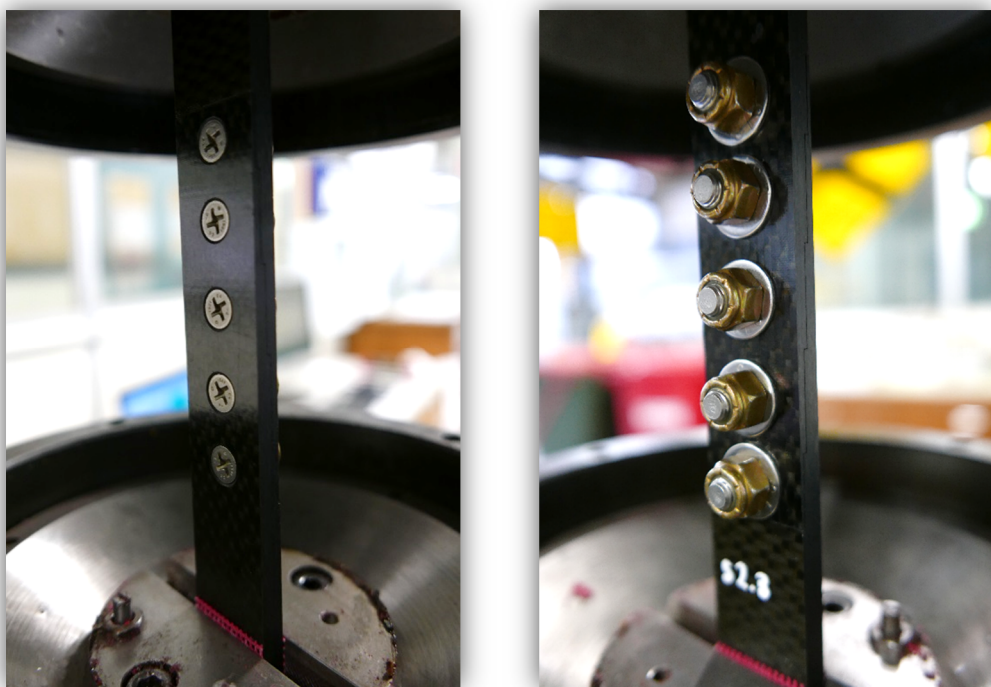
Figure 6.3 Configuration 2.2 - Bolted step lap joint configuration with five fasteners
