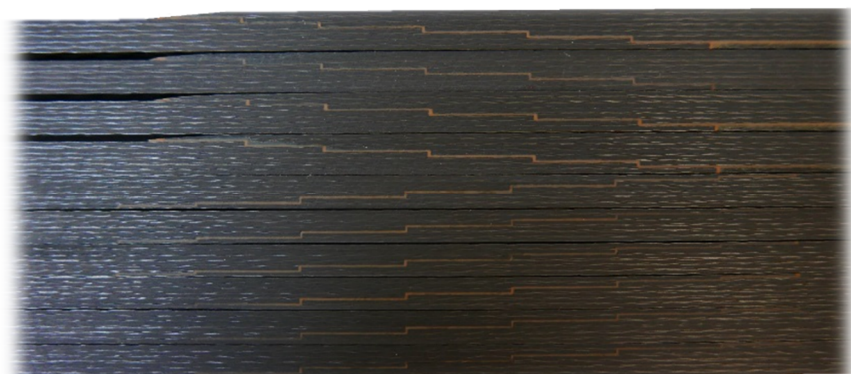
Figure 8.18 Bonded step lap joint configurations cured in an autoclave at 121°C for 90min; Configuration 4.1 - top; Configuration 3.1 - bottom
