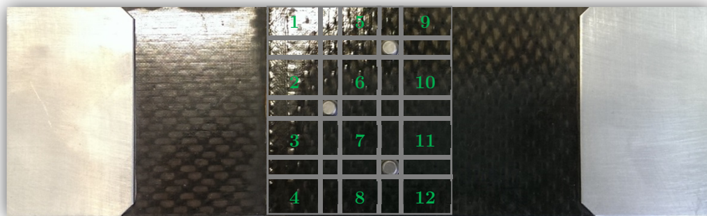
Figure 3.19 Ultrasonic scanning positions for Hybrid Configuration 1.4
