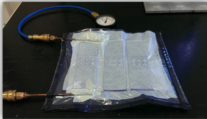
Figure 3.16 Vacuum bagging hybrid double lap joint specimens to cure bondline in an autoclave
