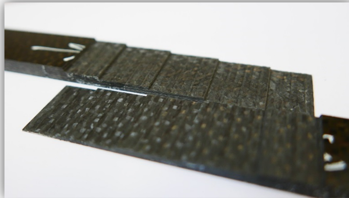
Figure 3.12 Thick HexPly M18/1/G939 carbon fibre adherends machined using an NC machine
