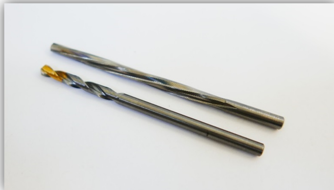
Figure 3.13 Solid carbide drill bit and reamer used for rivet holes in Stage 1
