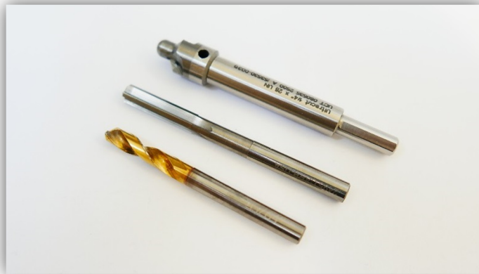
Figure 3.14 Solid carbide drill bit, reamer and countersink used for the countersunk bolt holes in Stage 2
