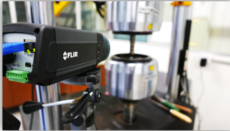
Figure 2.19 Non-destructive inspection using a FLIR A615 thermal camera
