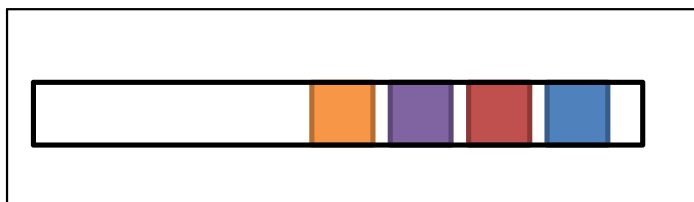
Figure 14: An example of a multiple-analyte 1D paper diagnostic on a dipstick.
