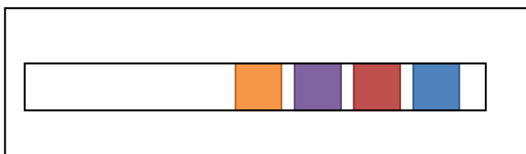
Figure 4: Example of a multiple-analyte 1D paper diagnostic on a dipstick.
