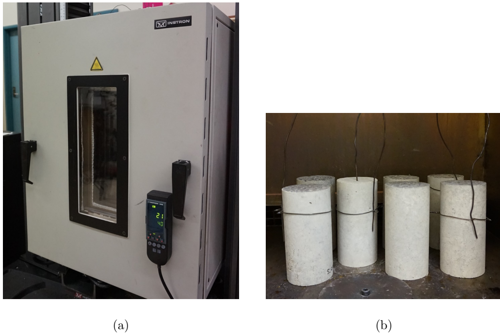
Figure 6.3: Laboratory setup for temperature exposure. (a) Environmental chamber and (b) placement of samples in groups of 7 inside the chamber.
