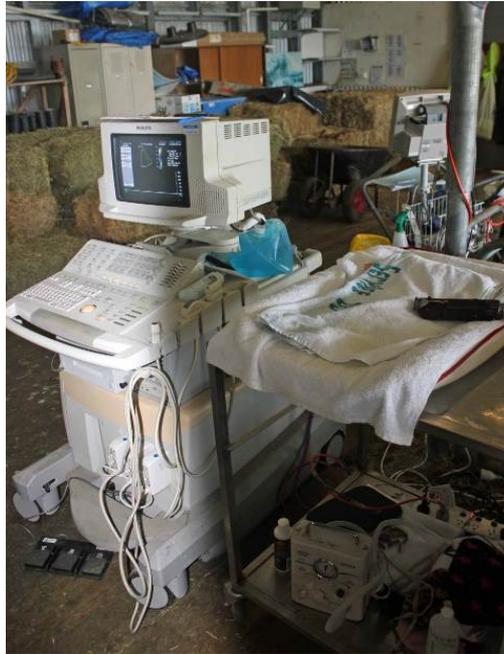
**Figure 2-2: Philips ATL SonoCT® ultrasound system set up next to a table for scanning lambs up to two weeks of age.**
