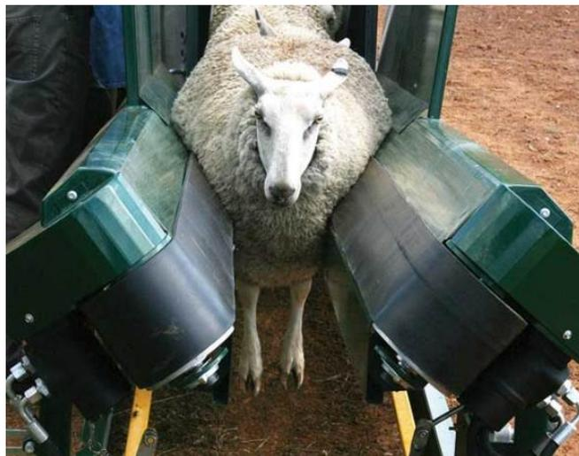
**Figure 4-6: An adult sheep on a V-drive being held securely above the ground by rubber belts that can transport the sheep forward and backwards.**
