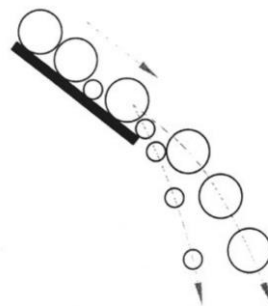
Figure 2-2 Trajectory Segregation (Silva et al. 2000)
