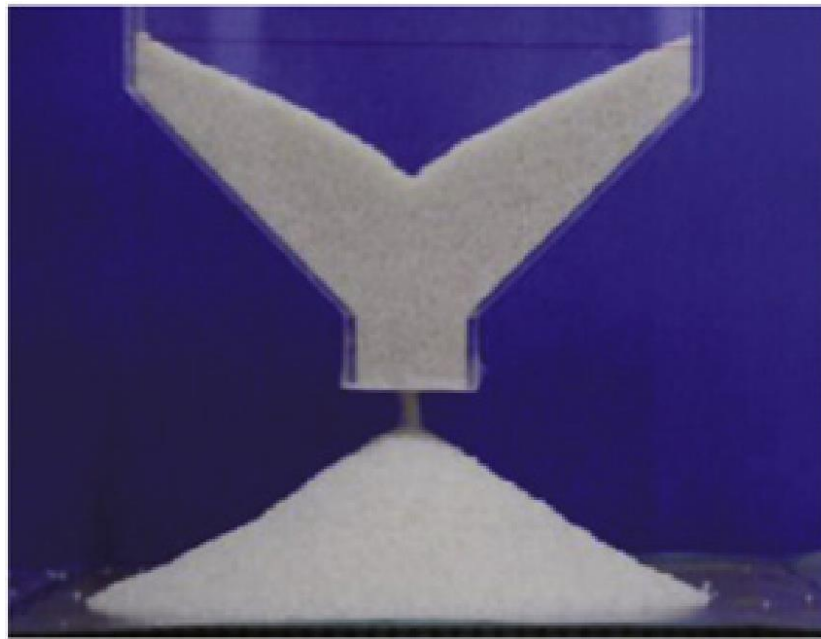
Figure 2-9 Formation of a sandpile as grains flow from a funnel onto the flat surface
