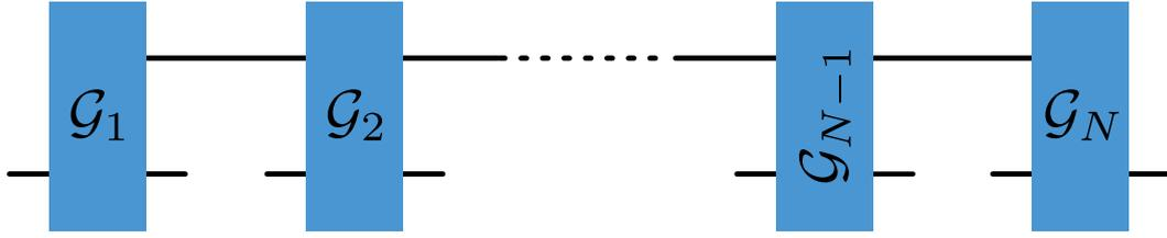
**Figure 5.12:** Concise dilation of an open process. By absorbing the initial state and the final trace into the respective CPTP maps, every open process can be represented as a sequence of CPTP maps  $\mathcal{G}_\alpha$  (under the assumption of an initially uncorrelated system-environment state). Once these maps are known, all joint probability distributions can be computed.
