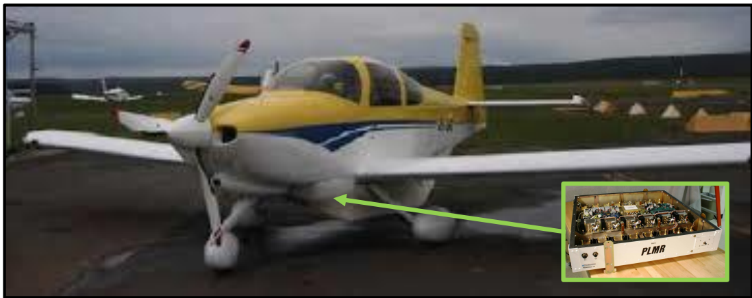
Figure 3.3: The aircraft equipped with PLMR L-band passive microwave instrument.
