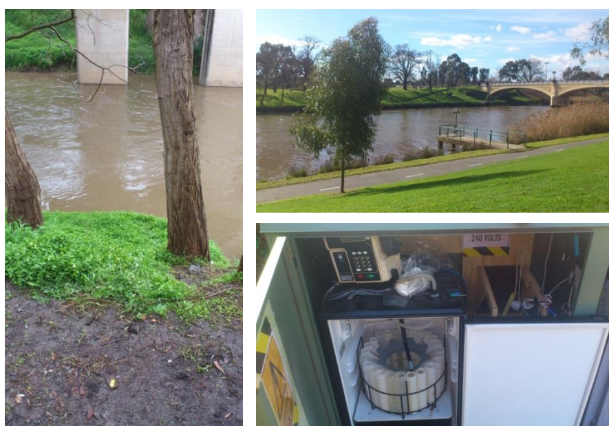
Figure 3 - 2 Left – Abbotsford monitoring site – sample intake point below the bank; Top right - Morell Bridge monitoring site (sample intake and top EC/T measurements point is at the end of the fishing pier); Bottom right – sampling stations setup.
