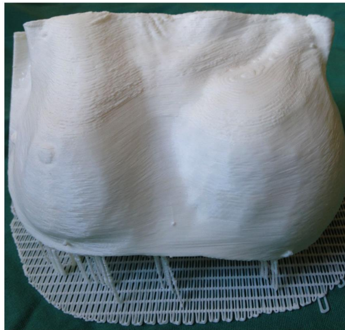
Figure 12.3.2.1.5. A three-dimensional (3D)-printed haptic, tactile biomodel of the breasts, produced from computed tomography (CT) data. Printing performed with the Cube 2 printer (3D Systems, Rock Hill, SC, USA) using Cubify software (3D Systems), and using white polylactic acid (PLA) filament ink.
