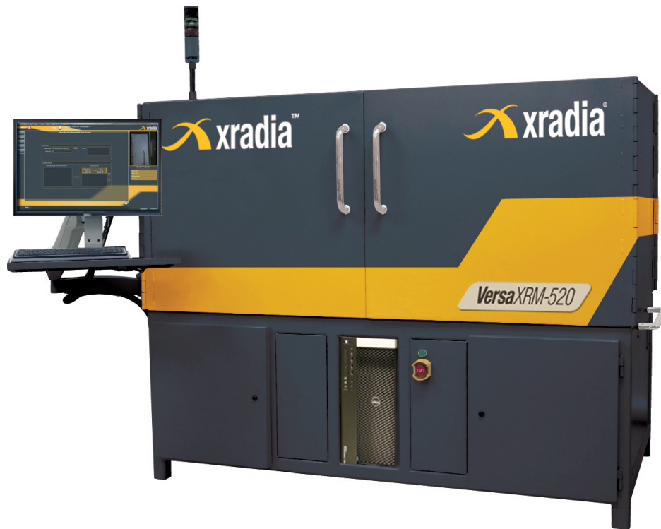
Figure 3-1: X-Ray CT machine housed in Geomechanics Laboratory of Monash University
