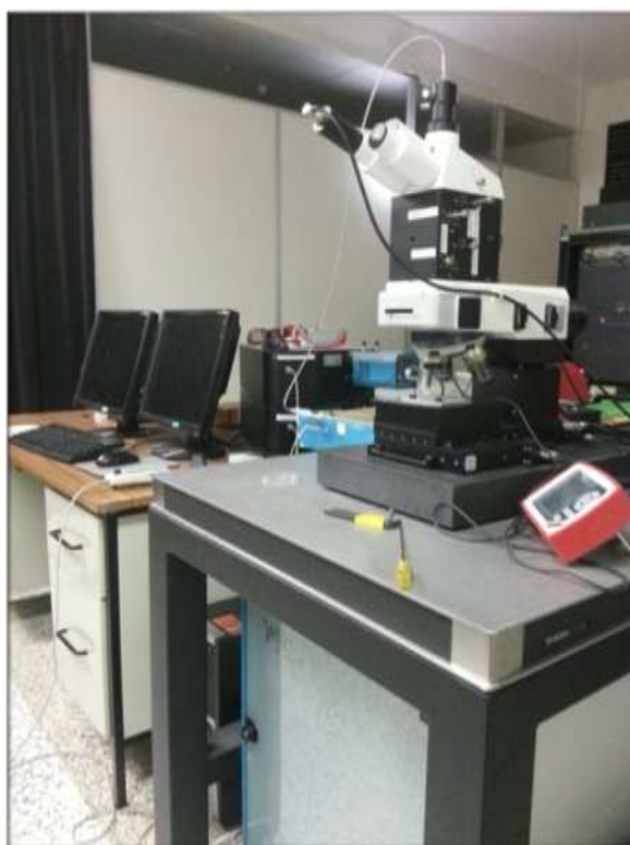
Figure 4.4: The WITec alpha300 R confocal Raman microspectroscopy in the spectroscopy laboratory of School of Chemistry, Monash University.
