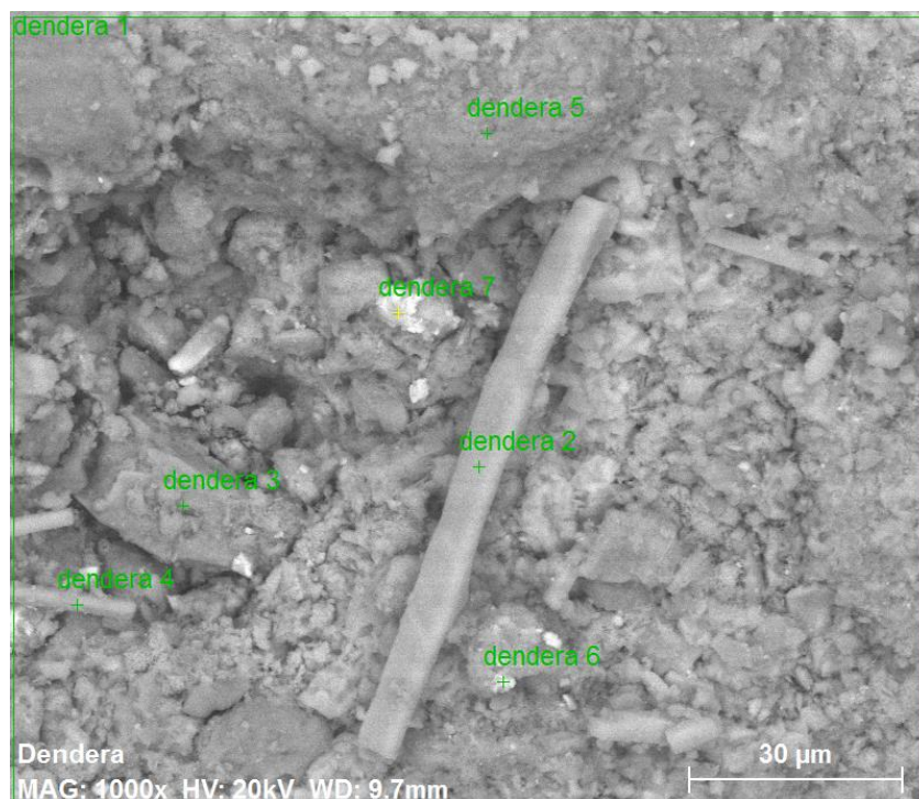
Figure 5.51. Nova, BSE image showing the Points of Interest as marked, blue region within Dendera sherd DE 1. More of these long rod-like particles were observed spread widely over the entire blue pigmented region. Gypsum is both on the surface of these particles and crystals of gypsum were located. Again, the source of these particles is unknown, but it is likely to be from an organic source such as plant material.
