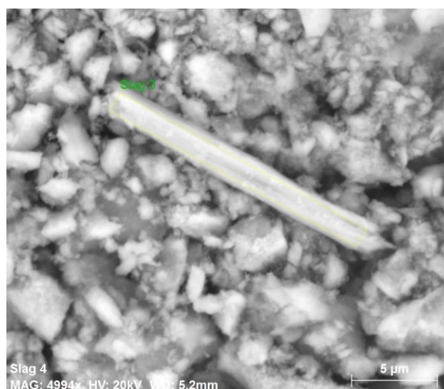
Figure 5.6. Image of high iron particle within the core of the Mut al Kharab slag sample.
