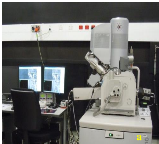
(a) FEI Quanta 3D FEGSEM™ Focussed Ion Beam electron microscope (Monash Centre for Electron Microscopy)
