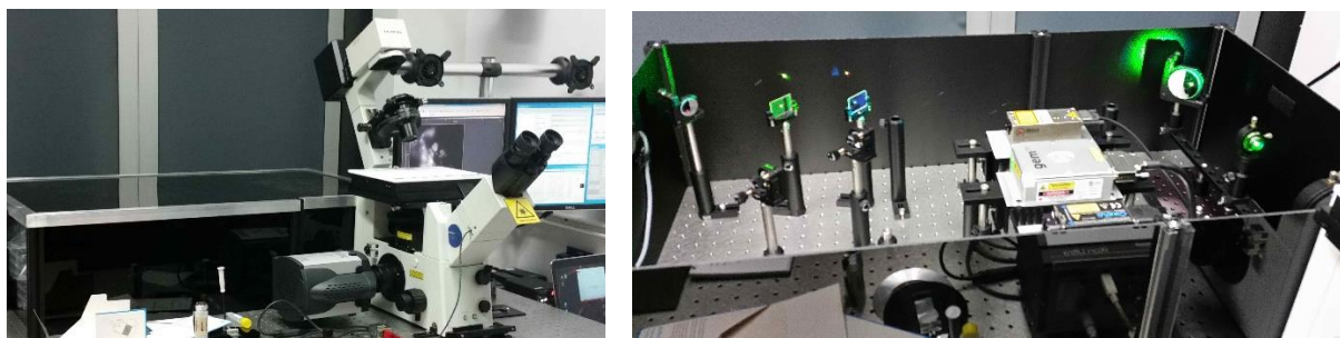
Figure 2.1 Custom build d STORM set-up at Monash Micro Imaging facility. The set-up includes Olympus IX-71 base (left image) equipped with the appropriate fluorescence filter cubes (right image) and a high speed EMCCD camera with single photon sensitivity for single molecule detection.
