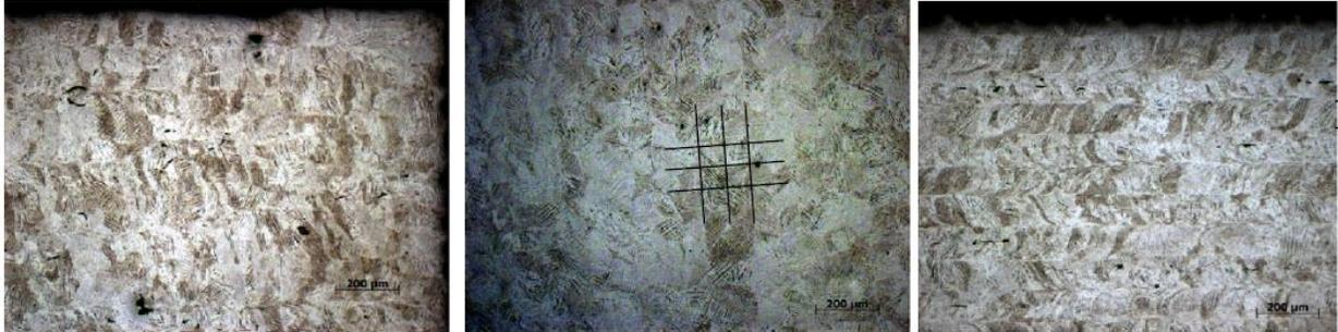
**Figure 2-24 From left to right: top-view microstructures of unidirectional scanning strategy, cross-hatching scanning strategy, zigzag scanning strategy [24].**
