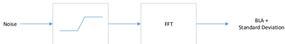
Fig. 3-1. Illustration of noise excited BLA of nonlinear system
