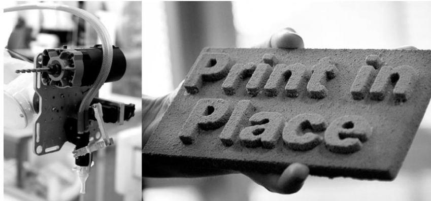
Figure 2-10 Combining additive and subtractive processes in the Print-in-Place construction method
