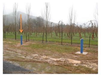
**Description and Comments:** Bore located on Harris Lane close to junction with the Buckland Valley Rd. **Continuous Data:** Continuous water depth and electrical conductivity data are available for this site, measured with InSitu AQUA TROLL 100 at 30 minute intervals.
