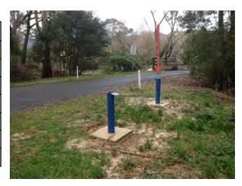
**Description and Comments:** Bore located close to the bridge (west side) on Harris Lane. **Continuous Data:** Continuous water depth and electrical conductivity data are available for this site, measured with InSitu AQUA TROLL 100 at 30 minute intervals.
