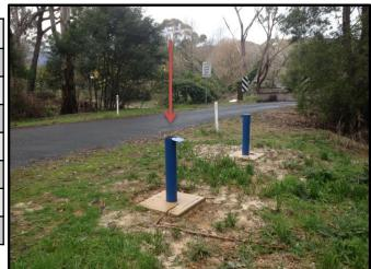
**Description and Comments:** Bore located close to the bridge (west side) on Harris Lane. **Continuous Data:** Continuous water depth and electrical conductivity data are available for this site, measured with InSitu AQUA TROLL 100 at 30 minute intervals.
