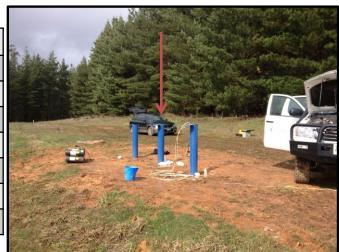
**Description and Comments:** Bore located on Eggleston Lane near junction with Kennedy Rd. **Continuous Data:** Continuous water depth and electrical conductivity data are available for this site, measured with InSitu AQUA TROLL 100 at 30 minute intervals.
