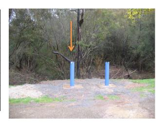
**Description and Comments:** Bore located close to the bridge (north side) on River Road. **Continuous Data:** Continuous water depth and electrical conductivity data are available for this site, measured with InSitu AQUA TROLL 100 at 30 minute intervals.
