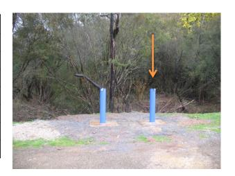
**Description and Comments:** Bore located furthest from the bridge (north side) on River Road. **Continuous Data:** Continuous water depth and electrical conductivity data are available for this site, measured with InSitu AQUA TROLL 100 at 30 minute intervals.
