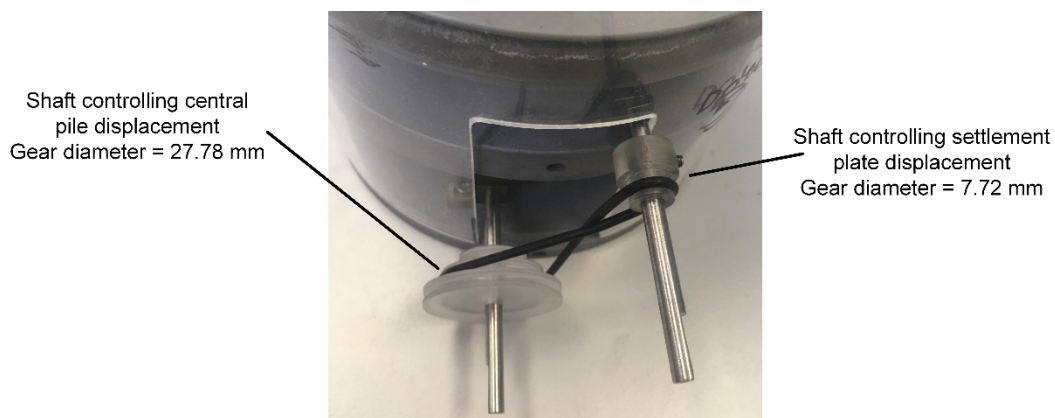
Figure 3.5: Gears and belt controlling the settlement plate and the central pile displacement.
