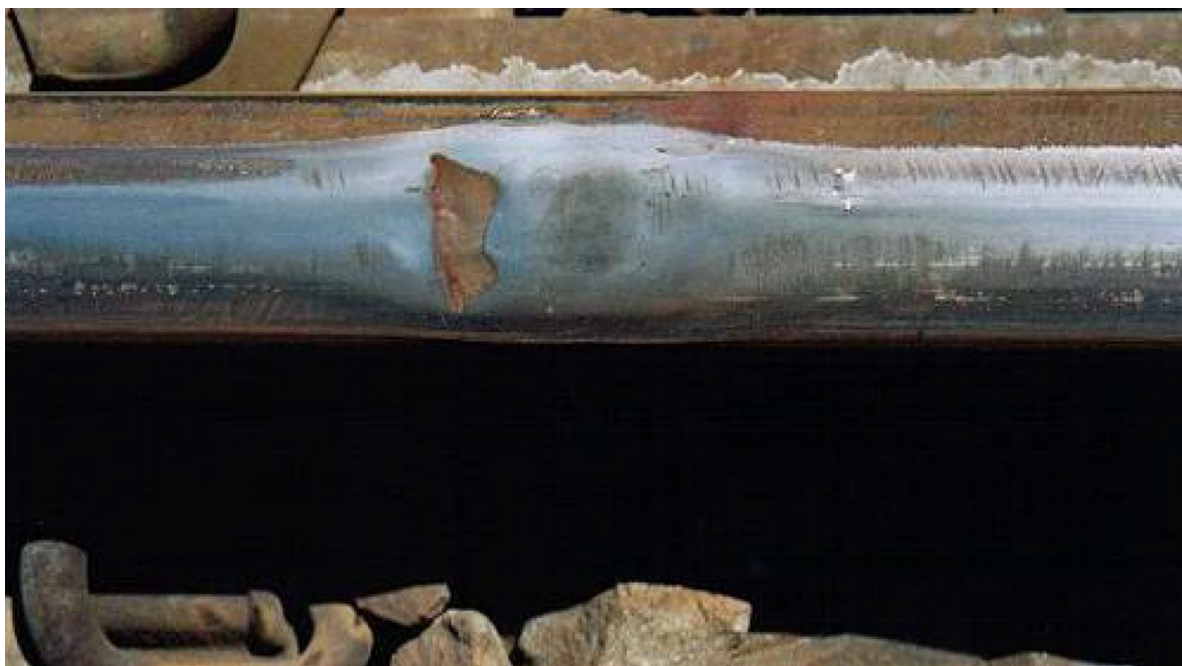
Figure 2-24 Severe stage of running surface squat. [1]
