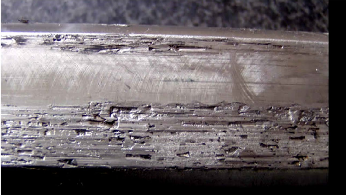
Figure 2-1 Abrasive wear (scratches) on rails. [2]
