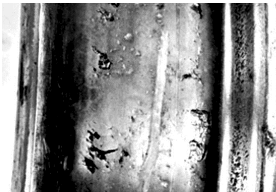
Figure 2-8 Wheel with surface fatigue mechanism. [2]
