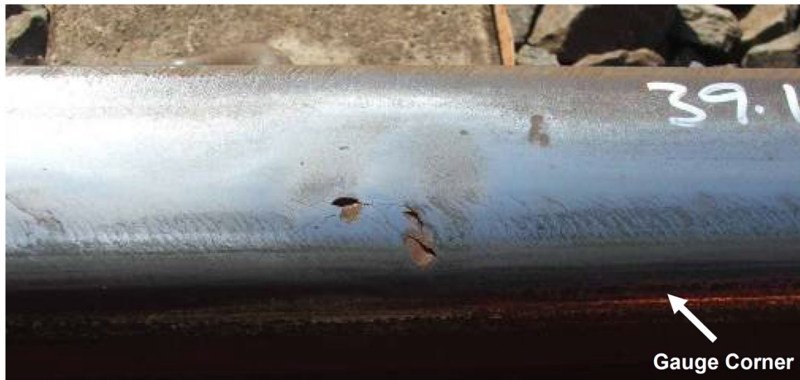
Figure 2-27 Severe stage of squats initiated by gauge corner checking. [1]
