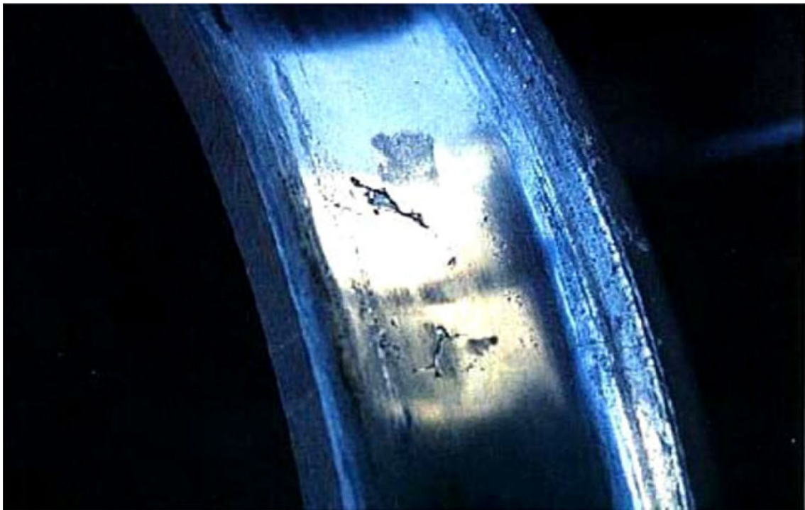
Figure 2-4 Delamination wear of wheels. [2]
