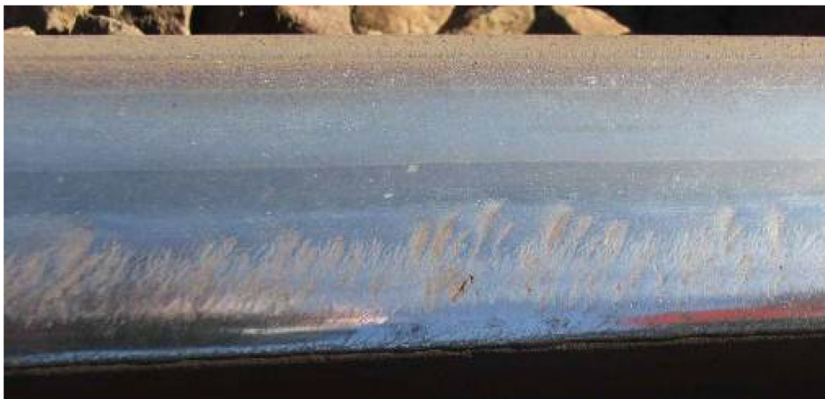
Figure 2-26 Intermediate stage of squats initiated by gauge corner checking. [1]
