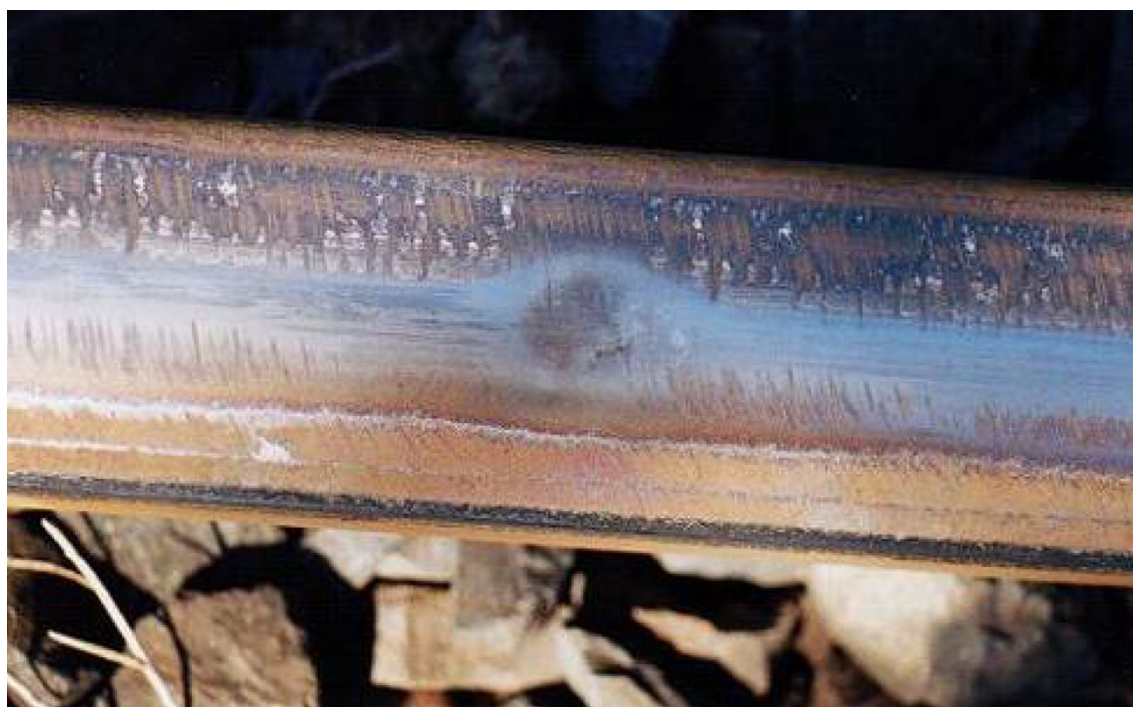
Figure 2-22 Initial stage of running surface squat. [1]
