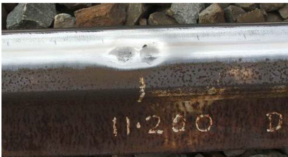
Figure 2-23 Intermediate stage of running surface squat. [1]
