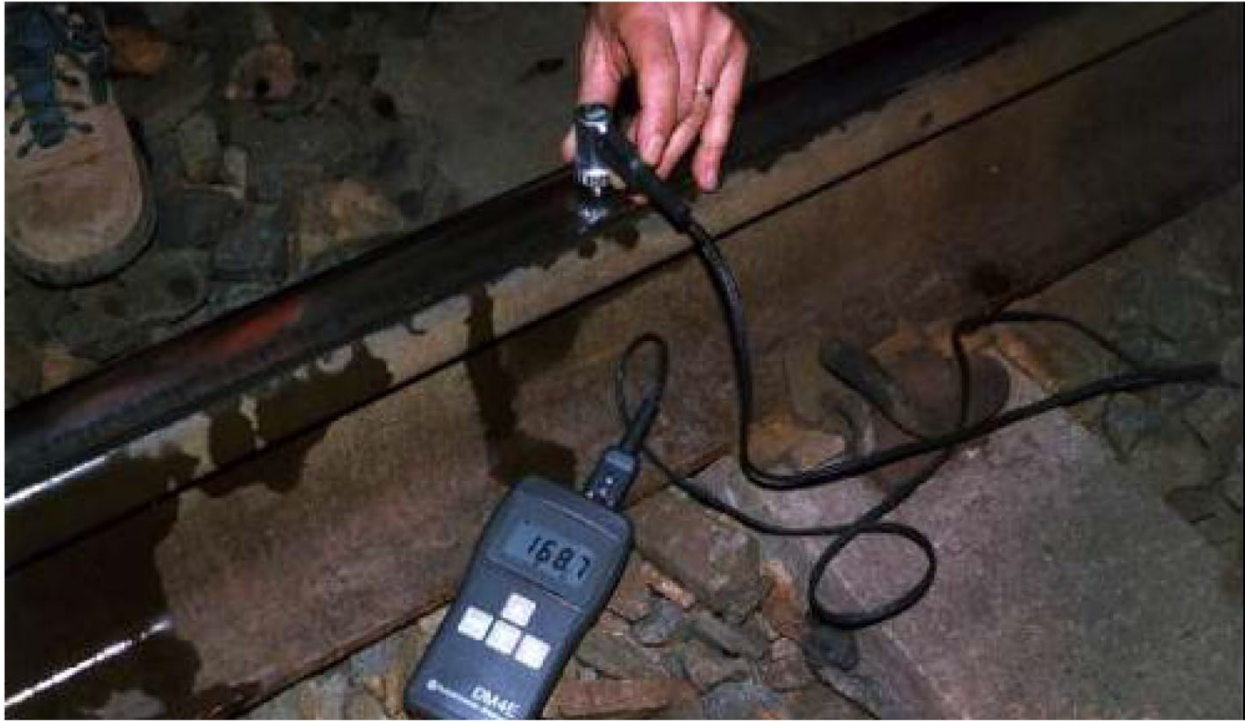
Figure 2-32 Inspection to determine the length and depth of subsurface squat cracks using an ultrasonic depth gauge. [1]
