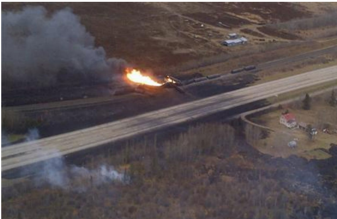
Figure 2-9 Train derailment in the town of Gainford, Alberta, Canada owing to surface defects.
