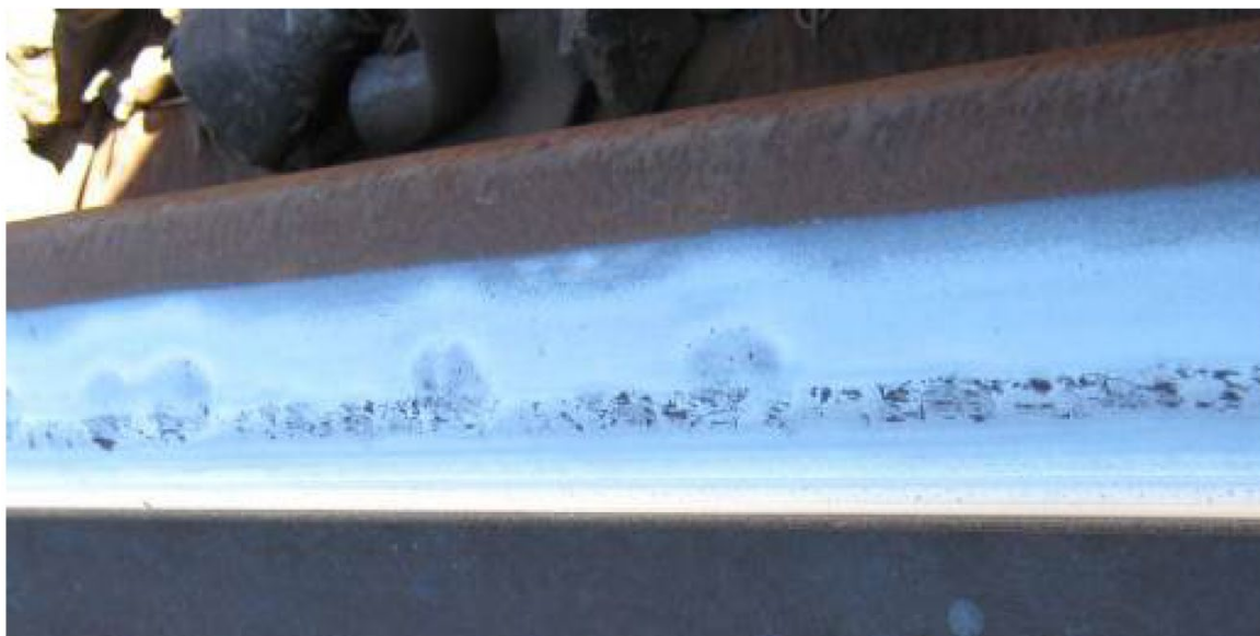
Figure 2-29 Running surface squats initiated from wheelslip. [1]
