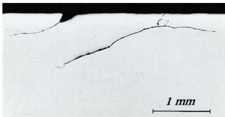
Figure 2-12 Cracks and spalls in initial stages develop in a rail longitudinal section. The crack propagates into the railhead and then level out. [1]
