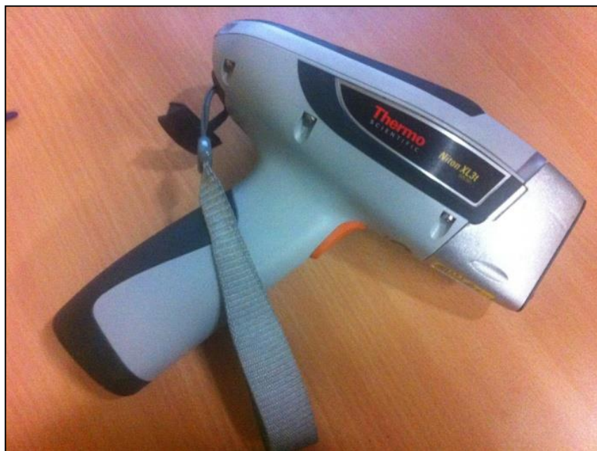
Figure 3: Portable X-Ray Fluorescence analyser used in this research.
