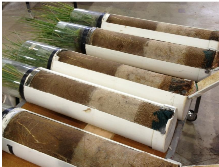
Figure 5.2. Partial removal of the biofilter column casing allowed visual inspection of the filter media and root architecture.
