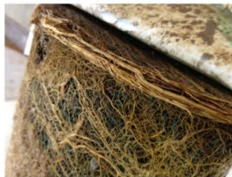
Fig. 3. Dense root growth at the column base was more extensive in the saturated zone-inclusive biofilters.
