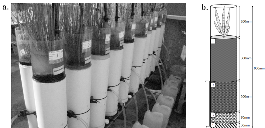
Figure 2.1. (a) Experimental set-up of columns in greenhouse (b) Schematic diagram of the biofilter columns (with saturated zone riser outlet attached)
