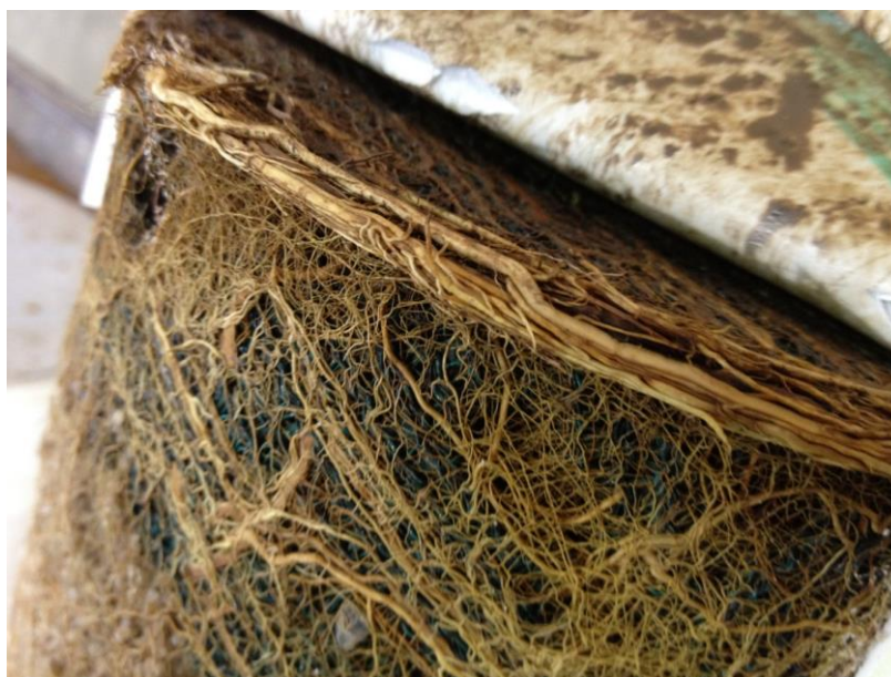
Figure 5.3. Dense root growth at the column base was more extensive in the saturated zone-inclusive biofilters.
