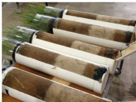
Fig. 2. Partial removal of the biofilter column casing allowed visual inspection of the filter media and root architecture.
