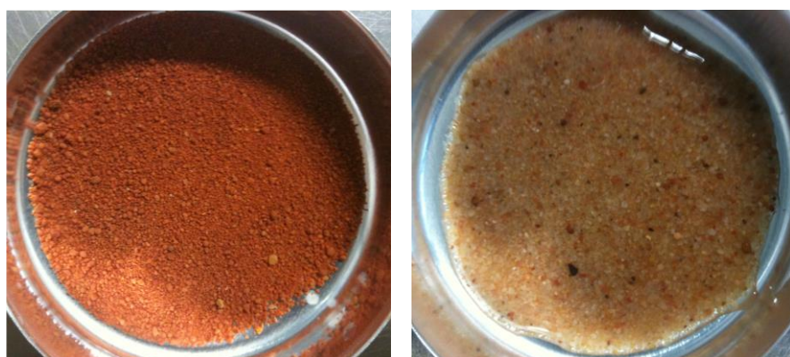
Figure 3.3. Skye sand before (left) and after (right) washing with a 0.1M NaOH solution and rinsing through a 100 \mu m sieve (wet).
