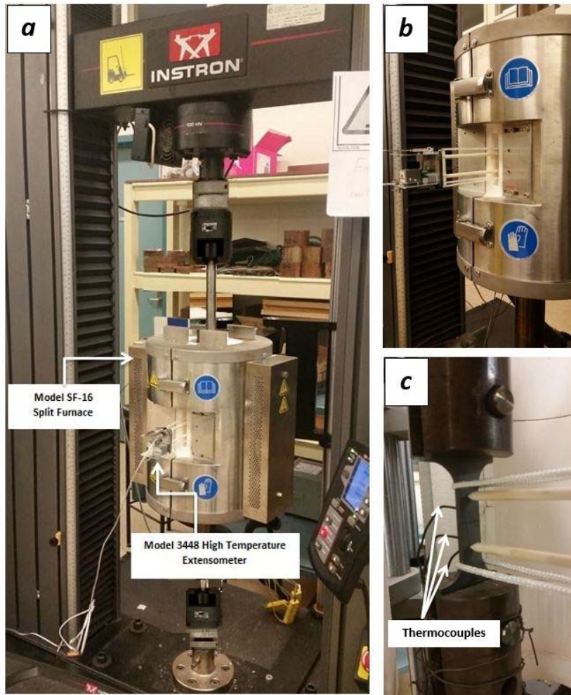
Figure 3-3. a and b) Test setup from different views, c) inside the furnace
