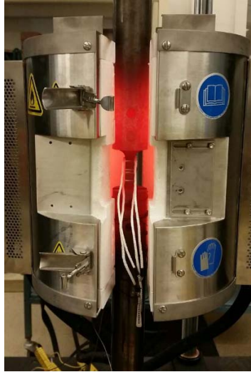
Figure 3-4. The cooling test setup for the post-fire stage ( T_t=800^{\circ}\text{C} )
