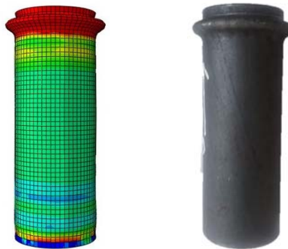
Figure 7-11. Comparison of the failure mechanism of the experimental and FE Model for UHSS-QT stub column cooled from 470°C to room temperature
